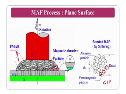
So, for planar surfaces whatever you have seen in the previous slide also is the planar surfaces, and workpiece is there, flexible magnetic abrasive brush is there, this is you can see clearly the North Pole and South Pole; where you have the magnetic abrasive particles are embedded. In this one and this field of lines will support the abrasive particles.
