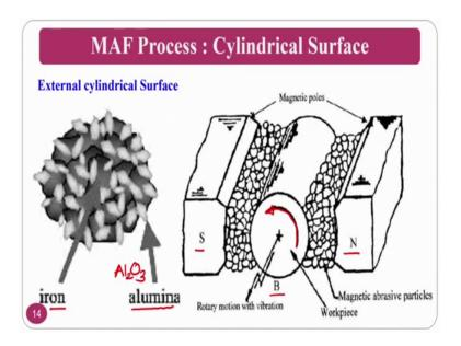
So, whenever you are going to use, the previously you have seen it is for the flat surfaces. Now if at all I want to see for a cylindrical surfaces. How it look like? So now, the cylindrical surface, you I have the South Pole, I have the North Pole, and field of lines will transfer always between North to South, ok. And you have the workpiece.
