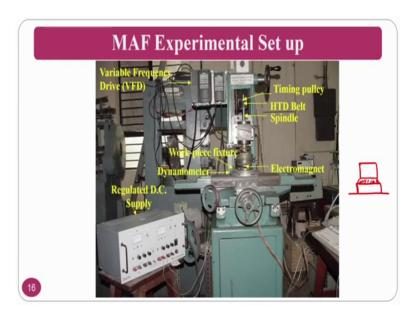
Because we fought all we want to understand the physics of the MAF process then we have to go for the simple surface to be finished. So, in this particular case, what we are going to see is the flat surface. How to finish is a flat surface where in the surface roughness is there. So, you can see here the electromagnet, the workpiece is there as well as the dynamometer is also there.
