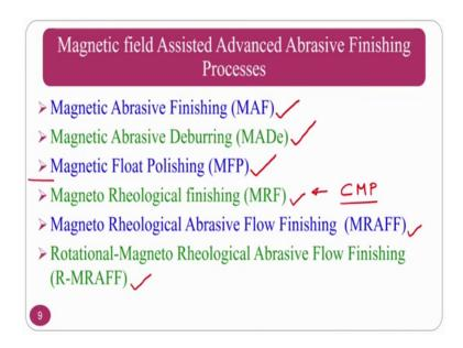
So, what we are going to study in this particular section of magnetic field assistant finishing process? We are going to study Magnetic Abrasive Finishing, Magneto Abrasive Deburring, Magnetic Float Polishing.
