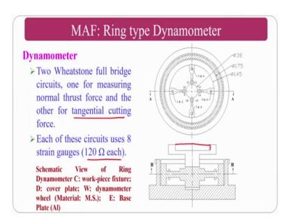
So, as I said dynamometer also used here; the dynamometer is a ring type dynamometer to wheat stone full bridge circuit one measuring the normal thrust force and another one measure the tangential cutting force. Each the circuit has 8 strain gauges. Normally, this as the strain gauge type of thing; so you can place the workpiece and you can measure
