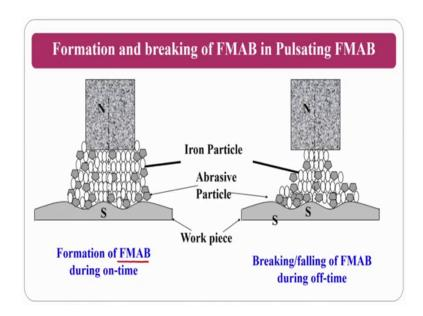
If you see here, the formation of flexible magnetic brush is constant in this one, but if you see the in terms of the static one, your chain is fix. That mean, that chain formation will be always there. So, that abrasive particles have or their embedded in the chains. But in the pulsating one what is the beauty about it one? You are giving a pulse then again you are giving a power.
