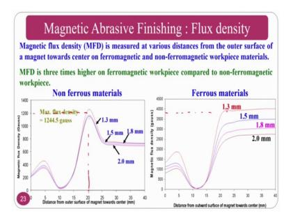
Magnetic abrasive finishing where you see the flux density magnetic, flux density is measured at various distances from the outer surface of the magnet, towards the centre of the ferromagnetic and non-ferromagnetic materials. So, magnetic flux density, 3 times higher in ferromagnetic work piece compare to non-ferromagnetic work piece.
