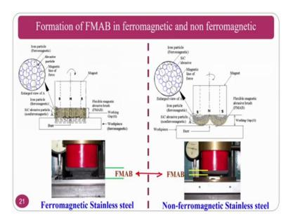
In the difference between ferromagnetic and ferromagnetic material, you can see here flexible magnetic abrasive brush is very strong in case of ferromagnetic, but not in case of non-ferromagnetic. And there will be adherence formation in the ferromagnetic, but it not in case of non ferromagnetic. But both the cases depend on your application you have to use this particular process.
