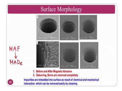
And you can see clearly the surface, the burrs formation and later it can be removed by the magnetic abrasive finishing process and particularly, it is for the deburring application. What I mean to say is magnetic abrasive finishing is used in this case for the magnetic abrasive deburring operation that is why this particular process is called magnetic abrasive deburring ok. Another process that we are going to see in a introductory way is magnetic float polishing ok.
