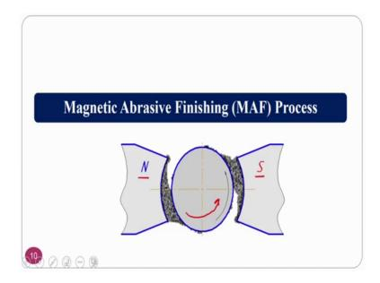
So, you can see here magnetic abrasive finishing process; where the workpiece is rotating continuously, and the abrasive particles are placed, where you have a North Pole and you have a South Pole. And the chains will form from North Pole to South Pole because of the rotation of the work piece. And other things the shearing action takes place and the material will be removed in a nanoscale or sub nanoscale and the surface finish is achieved in the nanometric range.
