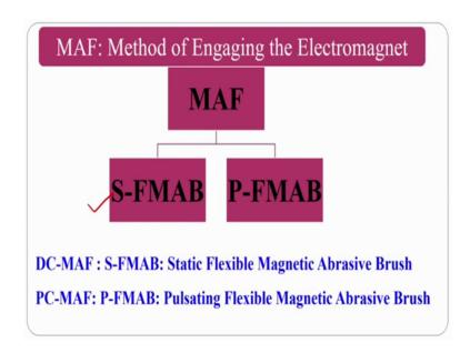
So, magnetic abrasive finishing process you have 2 varieties of flexible magnetic abrasive brush. One is static flexible magnetic abrasive brush; another one is pulsating flexible magnetic abrasive brush. In the static flexible abrasive brush what is happening is that whatever you have seen till now all will come under the category of static one ok. Because you are power supply, DC power supply is constant and you are going to get a static one.
