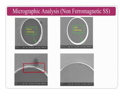
You can see the complete hole after drilling process, and you can have the burrs on the surface. The drilling can be done by idiom process also, and idiom also can create a recast layer and the corresponding burrs also ok. It is not only the burr formation is not only specified for the conventional, it is also for the advanced machining processes also.
