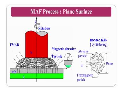
So we will use the similar setup. That is, MAF process for the plane surfaces only we will use, because we want a plane surface for that only requirement is that you have to remove the burrs so that you will get a flat surface.
