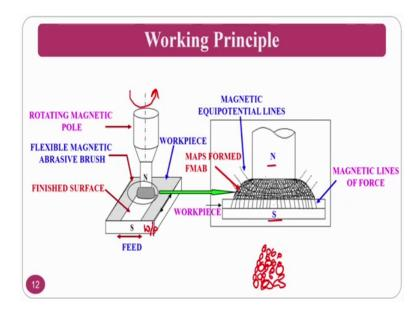
You can see the working principle, this is the feed is given to the workpiece, this is the workpiece, and the tool is there rotating magnetic pole plugs, and you have a flexible magnetic brush. You can see the North Pole is there, South Pole is there, where in your work piece is there. And you will form a magnetic field of lines that is not you nothing but you form the chains. So, these chains are formed and abrasive particles are entrapped, ok.
