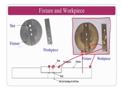
Instead of going for a big workpiece, we are making a slot in between, in case of magnetic abrasive finishing; we can finish this particular complete one ok. But if at all I want to remove the burrs on the flat surfaces, what I am going to do is that we are going to place the holes drilled surface. This is my work piece or this is my work piece, wherein I am going to drill a hole or setup holes I am going to drill, and this hoes will have the burrs ok.
