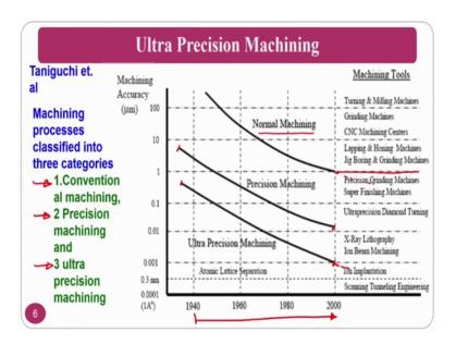
So, ultra-piston machining if you see the Taniguchi et al, they has given a table where the machining processes are classified into 3 categories. One is the conventional machining, second one is the precision machining, and the third one is ultra-precision machining; if you see that machining accuracy versus number of years are the as the time passes.
