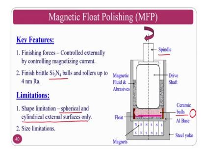
So, magnetic float polishing process, if you see the magnetic float polishing process, the magnetic poles arranged into North-South South-North like this. At the same time, you have the workpiece materials is a ceramic balls, and you have the magnetic fluid. You are going to have the spindle and these are the ceramic balls these are the spherical balls.
