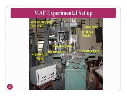
For the same as I said we are going to use the same experimental setup that we have seen in the magnetic abrasive finishing process. And the slight change that we are going to do is that we are changing the fixture.
