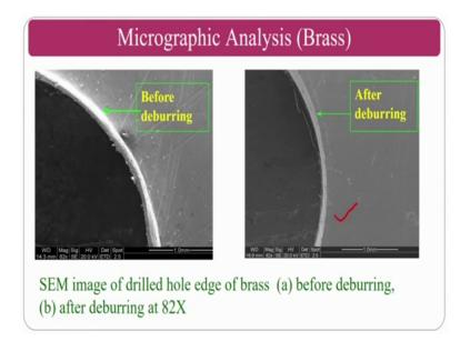
You can see some of the burs that are not removed from the drilling hole. These are the burrs before deburring operation. And after deburring operation you can see the there is no burrs on the flat surface ok.
