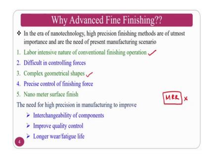
So, why advanced fined finishing process is required? Normally, this process is labor intensive methods, because the final operation that one can do on particular component or particular workpiece is finishing operation in a mechanical spectrum. So, you have to acquire the tolerances, you have to acquire the finishing and many things.
