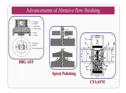
If time permits, we will see the advance versions of abrasive flow finishing process like drill bit guided, spiral polishing, centrifugal forces abrasion for from shearing process and other things also in upcoming classes subjected to if, the time permits ok. Thank you for your kind attention for this particular class and I am very thankful for various researchers for their figures and other things in the area of abrasive flow of finishing.
