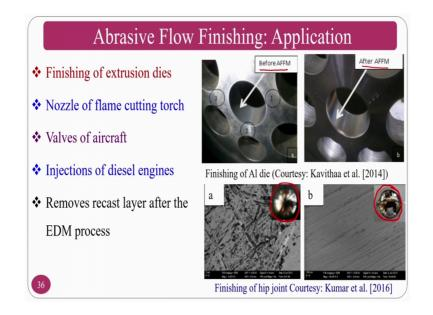
So, the applications finishing of extrusion dies, nozzle also can be done. Walls of the aircraft and it can remove the recast layers and other things, that can be done if you can see here before and after it is finished in a great level, at the same time you can see head
