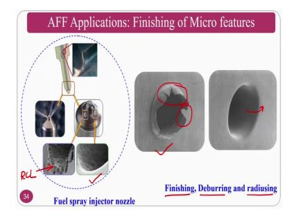
Normally, if you see the, you can do for the micro applications, the finishing of micro holes that are the fuel injector nozzles can be finished and this is the recast layer. This recast layer can be removed and it can be finished at the same time deburring. I was talking about in some of the cases deburring and other things exclusively I kept this particular slide for those people who could not understand: what is a deburring operation.
