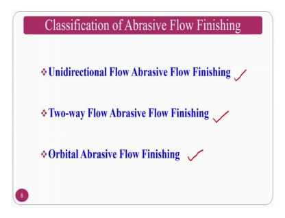
So, the classification of abrasive flow finishing process there are normally 3 varieties; one is unidirectional flow abrasive flow finishing process, two way abrasive flow finishing process and the orbital abrasive flow finishing process. Unidirectional abrasive flow finishing process also called as one way abrasive flow finishing process also ok.
