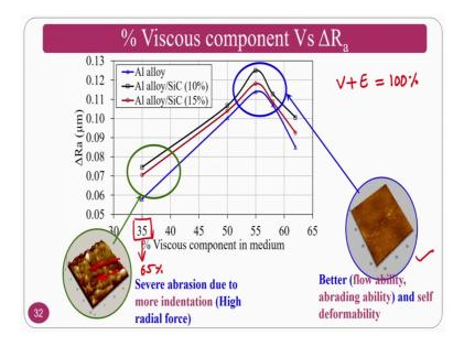
If you see the effect of rheology on the finishing of the medium if, you are going to measure your viscous component plus elastic component considered to be 100 percent in a visco elastic medium, if you are going to have 35 percent of viscous component. That means, that here so 65 percent will be your elastic component; that means, that elastic component is too high because of which it is not only shearing the peaks but also it is creating its own scratch marks.
