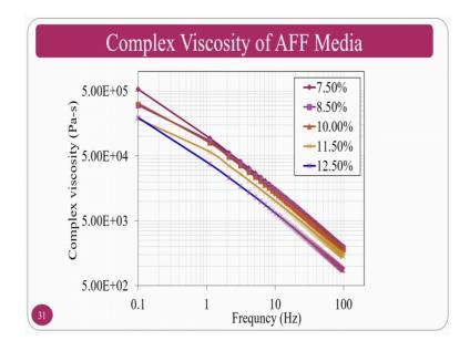
So, the complex viscosity of the medium if you are going to increase the frequency with respect to the time normally, this comes under dynamic. So, where the complex viscosity normal it can be measured or you can also measure storage modulus, loss modulus and tan delta other things also can be measured. If you are going to increase the frequency normally, the viscosity will gradually decreases because, the polymer chains will break and the viscosity will gradually decreases.
