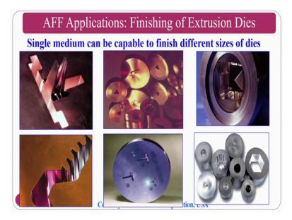
These are the extrusion dies various type of extrusion dies can be finished by the abrasive flow finishing process and you can also do the finishing of multiple holes in a die also that also is possible.
