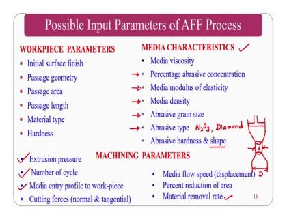
So, the work piece parameters initial surface roughness; initial surface roughness is very very important input parameter because, you cannot get a nano surface roughness, if your surface roughness is 100 microns or 200 microns. For example, if you are developed a hole using EDM process with carbon based dielectric fluid, it is damn difficult to finish into the nano. So, what you have to do is, your initial surface should be like 1 micron or less than 1 micron then, you can get the nano surface.
