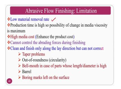
This is the advantages of this particular process. This process has limitation like low material removal rate. Production time is very high because, as you are going to increase the finishing time high the viscosity of the medium will go down. And medium cost is very high if, you at all you want to go for a commercial medium normally, the medium is too expensive. So, the production cost of your finishing component will goes up.
