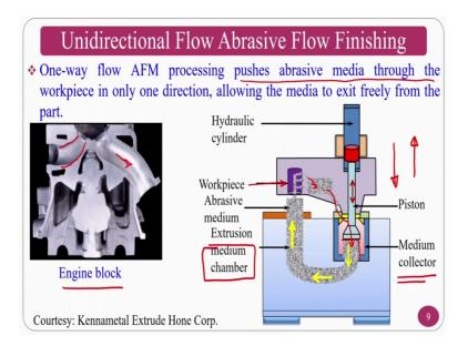
First we will see unidirectional abrasive flow finishing process where the medium is located in a medium collector. This one, this is a location and this is pressurized by using a hydraulic cylinder piston and the medium will pass through the extrusion medium chamber extrude through the workpiece ok.
