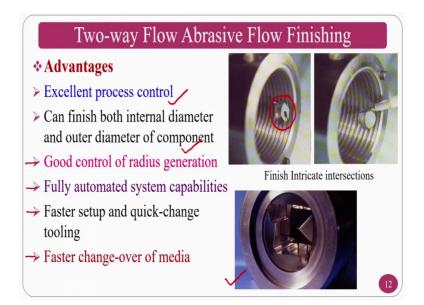
So, deburring action also can be taken place by using abrasive flow finishing So, the advantages is excellent process control will be there, can finish both internal diameter as well as outernal diameter. This will be depend on how you are going to develop the
