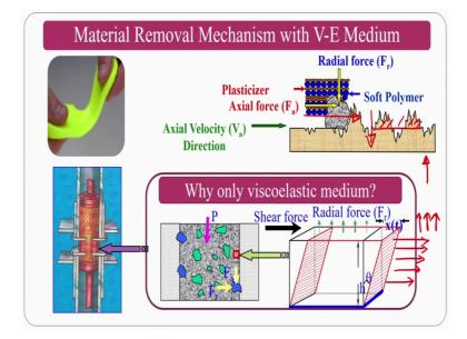
This is the mechanism that, we have seen and which we have not seen in the previous classes is, how the abrasive particle this particular abrasive particle is going to get the assistance of viscoelastic nature.
