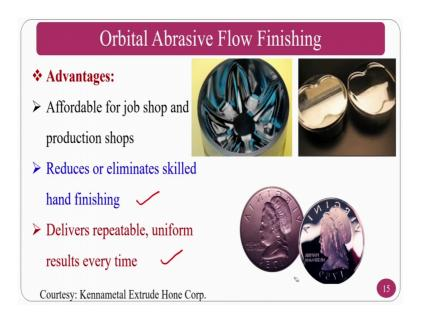
So, the simple to complex surfaces that one can finish using orbital abrasive flow finishing process is this. So, you can finish this type of dice you which are given, at the same time coins also you can do the finish ok.
