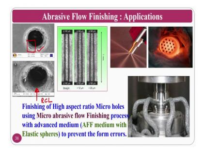
So, this is what I am talking about the recast layer. So, this is a laser beam machine surface, you can see the recast layer; that means, in a laser beam machining melting and
