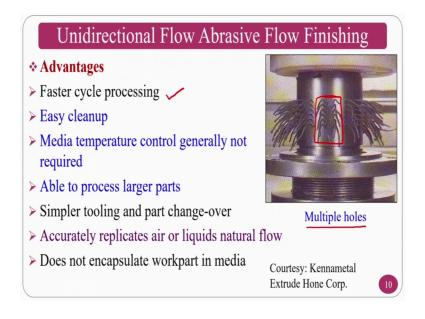
So, the another application of this particular process is, you do not require the medium collector and other things; that is called the multiple holes based work pieces can be finished. Multiple holes based workpieces where you will have a big medium cylinder wherein, the medium is filled and you are extruding through these holes. Whenever you try to extrude this one what will happen it is the one way so, the medium comes out through these holes and these holes will be finished properly.
