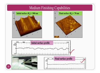
So, you can see the surface roughness as I said initial surface roughness is always important to understand and to get the nano surface finish in the later cases. So, initial surface roughness is 900 nanometers and the final surface roughness is 70 nano meters and the initial profile and the final profile you can see the mirror image of the pen tip in the workpiece ok. So, this is how you are going to finish these particular components.
