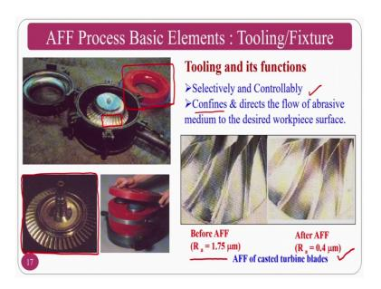
So, tooling and its functions if you see the selectively and controllability, that means that it has to select locations of the workpiece, so that the medium flow across that particular section only and controllability. So, it has to flow uniformly under the control of this particular friction and it should confine and direct a flow of abrasive medium across the cross-section to be finished, ok.
