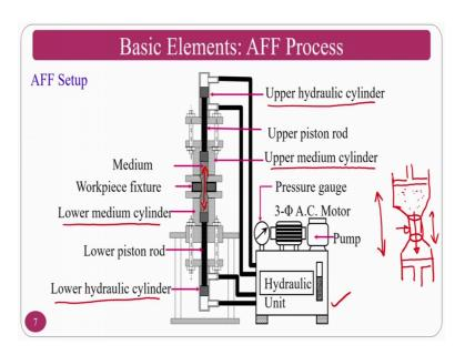
That means that it can we be used for fuel injector nozzles and others. Wherever the fluid flow is most important and fluid flow which is to be controlled or controlled fluid flow is required, there you can do the surfaces to the nano scale and you can achieve a better surface.
