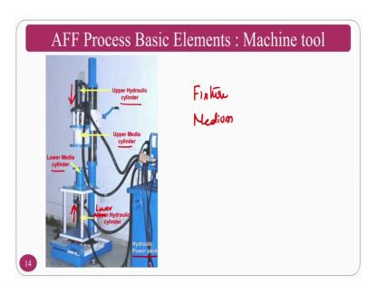
So, this is about the experimental original picture. Whatever you have seen in the previous slide is the schematic drawing. This is the experimental setup where you can see the lower medium cylinder, upper medium cylinder, upper hydraulic cylinder, lower
