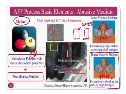
So, the medium, most important and critical component of this particular abrasive flow finishing process is nothing, but the medium, ok. So, the medium this is one what are the picture is taken from extrude hone which is now a days it is called Kennametal extrude hone. So, it will have the base polymers that is nothing, but visco elastic polymers with rheological properties and fine abrasive particles,.
