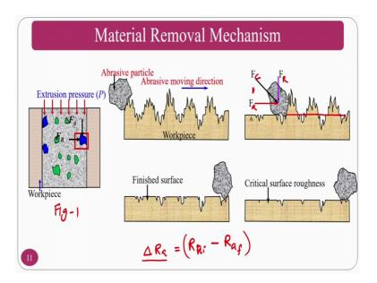
So, material removal mechanism which we have seen here, so viscoelastic nature is there and the abrasive particle as we have seen this is the abrasive particle where you are getting the assistance from the visco elastic polymers. So, visco elastic polymers if you see here, this is the axial force and this is the radial force and this is the resultant force,. Assume that I will say it is a cutting force or something, the resultant of this one, ok.
