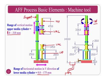
Abrasive flow finishing process basic elements, the first element is machine tool, ok. This is a machine tool drawing if you want to develop your own dimensions. Also given this is the laboratory scale development that is done and it has a various motions also, so that you can accommodate different size and shape component, ok.
