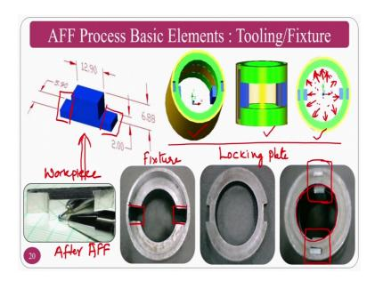
So, if at all I want to finish a flat surfaces, assume that this particular is my work piece and I want to finish it because see till now you have seen it is a cylinder and other bevel gears and other things what about the flat work pieces. You can also accommodate these things in a hollow cylinder. How to accommodate? If you see that you have the these type of work pieces.
