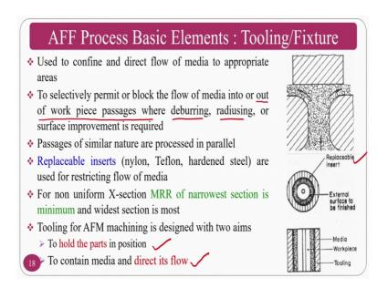
If you see here assume that I want to finish this particular component. So, I need to give the tooling as per the requirement, ok. So, used to confirm the direct flow of the medium appropriate area. That means that it has to guide the abrasive medium across the abrasive medium as I said this is semi-solid medium and it has to flow across the surface to be finished. When it will finish, if it can flow across the surface uniformly, then uniform surface finish can be generated, ok.
