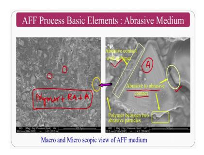
So, you can see the medium normally. So, the medium having lot of abrasive particles which are there in the polymer rheological abrasive medium, where you have polymer, where you have rheological additives and abrasive particles, ok.
