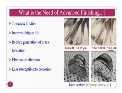
So, what is a need to reduce the friction it means that if you are going to get the micro to nano surface finish or you can reduce the friction improve the fatigue life.
