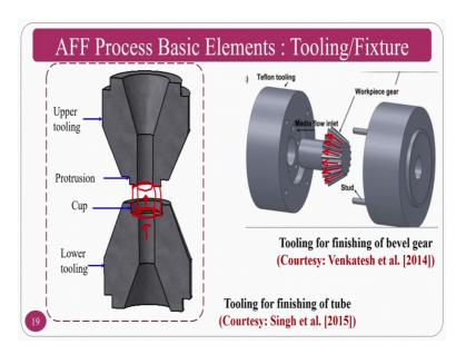
So, the tooling suppose I want to finish a cylindrical workpiece. For that purpose what normally you can do is, you can have a cylindrical workpiece and you can this can be a fixture and to understand make you to understand we have put this particular thing and this can be the outer diameter and this can be a inner diameter, ok.
