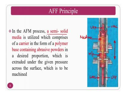
So, this in clear way I will show you the finishing region how it will take place. In this one, you can see here the medium is placed in the top medium cylinder. This is the medium and this is the upper medium cylinder, this is the lower medium cylinder.
