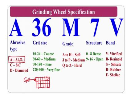
So, how do you specify, for example, let me take an example to explain a grinding wheel specification ok. So, A 36 M 7 V this is what the grinding wheel specification. A represent abrasive type; abrasive type means whether it is a alumina; that means, Al 2 O 3 or silicon carbide or diamond or something, ok. So, normally in this particular contest A represents 2 alumina, ok; that means, that my grinding wheel specification whatever I am asking having abrasive particles type is alumina.
