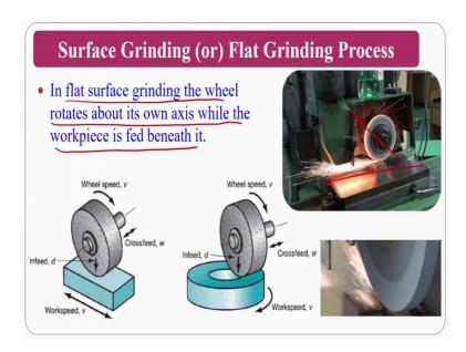
So, surface grinding normally it or the flat grinding you can go for wherever it is a parallel to the work piece surface. Flat surface grinding that the wheels rotate about its own axis while the work piece is fed beneath it this is called the flat grinding as you can see the work piece is beneath it for and this is my axis and this is my work piece axis, both are parallel to each other. This is called surface grinding.
