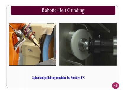
If you see whenever the implant is pressed against the grinding wheel what will happen? This wheels are made up of rubber bonding or this are elastically deformed, ok. If you can clearly see now the deformation of the grinding wheel is taking place that is called rubber bonding wheels or the soft plot best wheels they are going to use, ok.
