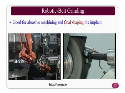
Here in this case you can see the robotic belt grinding where the belt is continuously moving and the knee implant is coming in and it is robot is giving its own motion. So, that it press against the grinding wheel which is a belt here and it will remove the material. At the same time soft wheels also can be used to polish, ok.
