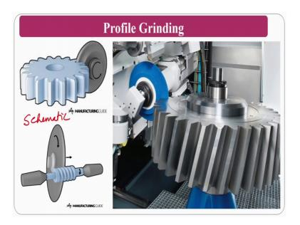
So, profile grinding also uses for making some the gears. As you can see the schematic this is the schematic diagrams and originally or practically if at all I want to see how the grinding process profiles are generated. Normally helical gates or spar gates all this type of gates also can be fabricated by the profile grinding. Only thing is that we require converse shape grinding wheels.
