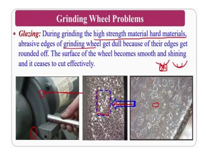
[FL] Grinding wheel problems first one is the glazing. What do you mean glazing? The glazing means for a practically what do you mean by glazing that thing is glazing; that means, it is shining.
