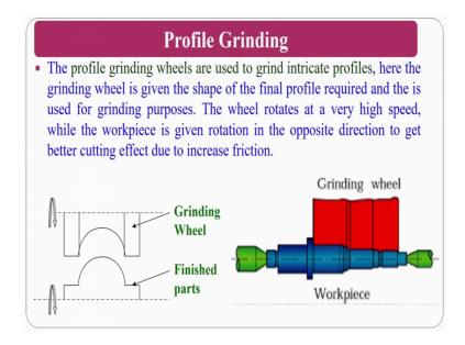
Profile grinding: if at I want to generate a profile in that circumstances you can generate or you can make a grinding wheel converse to it and you can generate. Profile grinding wheels are normally used for grinding intricate profiles assume that I want to do a work piece of this one or finished part of this one. So, the grinding wheel will be a converse shape.
