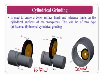
Cylindrical grinding whenever I am going to use the work piece here what normally the work piece is held in a rotatable jack and it can be rotated, so that the grinding wheel also
