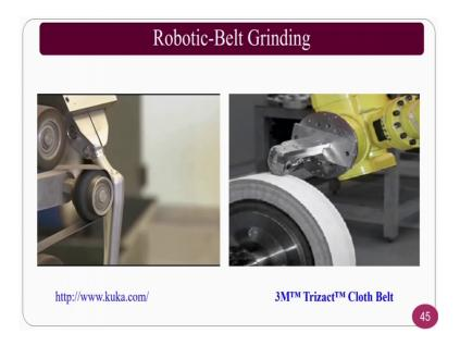
Robotic and belt grinding process. If you see the robotic and this is a costly process wherever if at all I want to go for finishing of complex surfaces, for example, here I am having a belt continuously moving belt is there.
