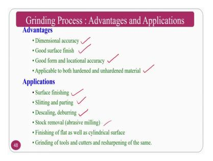
Advantages and applications; so, the dimensional accuracy will be very, good surface finish will be very good, good form geometry and local accuracy will be there and both hardened unhardened materials can be used, ok.
