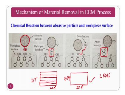
Mechanism of material removal, if you see the chemical reaction between abrasive particle, in the case one what is happening it has a water molecules which are there as a part of your abrasive slurry, this water molecule you have OH group and this OH at the same time work piece also on the surface of the work piece the abrasive slurry is moving.
