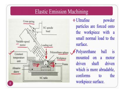
So, how the elastic emission works? If you see the elastic emission process, what will happen see, there will be a polyurethane ball here this is a polyurethane ball which is a tool basically on a work piece, and you can find there is a micron gap. There will be a micron gap with between your polyurethane sphere as well as a workpiece. This is flooded with abrasive particles which are very very fine in nature and along with the water or any other fluid ok.
