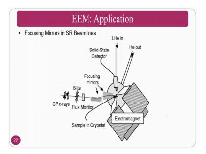
And the SR beam lines also if you see this SR beam lines are the mirrors focusing mirrors are machine by elastic emission machining process ok.
