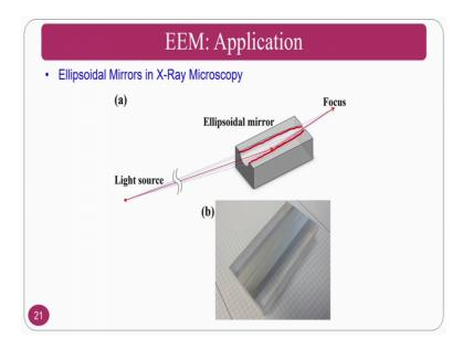
Ellipsoidal mirrors in X-Ray microscopy, you can do the finishing operation you can see there will be a gradual change in the curvature, and this curvatures can be machined by the elastic emission machining process.
