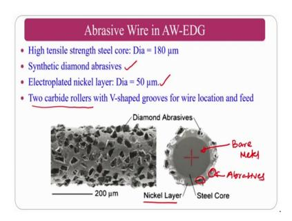
Abrasive wire basically it is a high tensile strength normally, if you see the abrasive wire how it look likes, normally it would should have high tensile strength because now this will have a carbide rollers with V shape and it will you need to have a tensile strength very good tensile strength because you have two spools which is rotating in the same direction. So, that the abrasive wire continuously moves and the tension between these two spools should be maintained constant.
