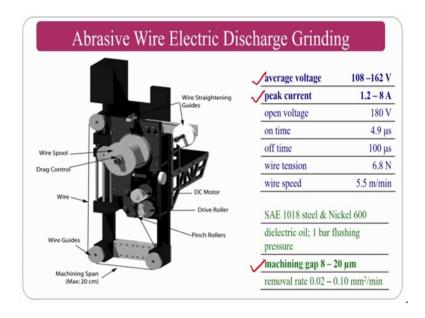
That is what is the advantage, if you see here this is how it also looks like wire E D M process only, but the thing is that here in the wire is having the abrasive particles. That current voltages are main important parameters here at the same time machine gap is also important factor which you can play in this particular process.
