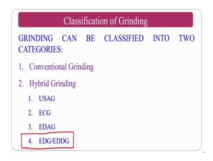
In the electric discharge grinding, grinding can be classified into Conventional grinding, Hybrid grinding. Hybrid grinding we have many things but in that particular class, we are going to see about electric discharge grinding and electric discharge diamond grinding process.
