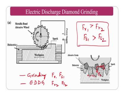
You can see here. So, how the material and other things are happening if you see the same mechanism here, what is happening here is the spark is taking place. If the spark is taking place this particular material will become melt and the thermal conductivity will pass on to this particular section and this particular section what will happen become the thermal is soften. So, the force required to shear, shearing force and the inertial radial force both are less compared to the grinding process.
