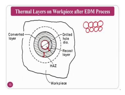
So, as I said that debris formation and other things. So, what you are going to see around the micro hole or the hole that developed using E D M process is this is my diametrical hole across it what is happening I said melting and evaporation ok. So, if there is a melting and evaporation if there is a spark because of the kinetic energy that is converted into thermal energy melting and evaporation, if there is a evaporation well and good if
