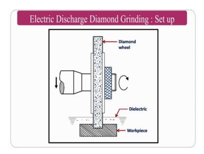
So, if you see the diamond grinding setup, normally the setup will be like this and dielectric fluid is fed at the same time the workpiece will be there inside, this is how you are grinding process looks like ok. Whatever you are seen in the previous one that is the machining region only of the electric discharge diamond grinding process in this one you can see the overview where you can give the negative terminal and positive terminal.
