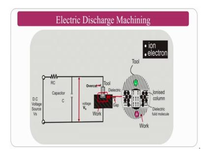
So, the electric discharge machining process if you see here, what will happen is this is a over view and I am going to tell you how the material removal mechanism will takes place and if you see this particular area is zoomed up here ok. So, the tool is given negative terminal and the positive terminal is given to workpiece and you can see here some of the things are ions some of the things are electrons how these are all will flow and the material removal mechanism will takes place.
