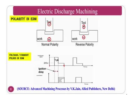
So, there are two Polarity one is the Normal Polarity and Reverse Polarity. So, normal polarity normally tool will be given negative terminal positive terminal will be given to the workpiece, in the reverse polarity some of the people they do the literature some of the people do the research on reverse polarity for electric discharge coating and other things people will say, in that circumstances people will use negative terminal to the workpiece and positive terminal to the tool ok.
