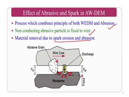
That is how it is the same explained in a close up view, this process combines a principle of wire E D M and abrasion non conducting abrasive particles are fixed on the wire; that means, that it will have the 2 D abrasion or the two body abrasion. The material removal due to spark erosion and abrasion that is called here what is your going to see here is erosion this is called the spark erosion and this is called abrasion ok.
