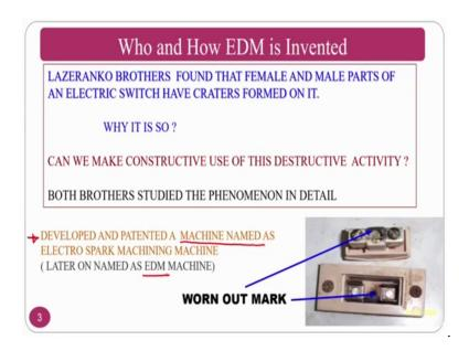
So, who and how E D M is invented. So, the LAZERANKO Brothers found that the female and male parts of an electric switch have craters formed on it. So, what will happen? So, whenever you see most of the in commonly houses if you see the electric connections have the switches where you have male and female part because of which if
