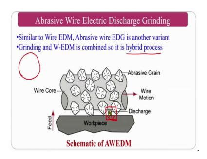
It is similar to wire E D M process, but abrasive wire E D G is another variant grinding and wire E D M is combination which is called as a hybrid process.
