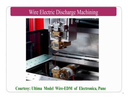
You can go for alumina and other thing that is why the word came at the start so; that means, abrasive wire electric discharge grinding process ok. So, before that we will just to see the wire electric discharge machining process this is the commercially available wire electric discharge machining process. You can see a wire here this wire will continuously rolling or it will be continuously moving by the spools and the material will be removed.
