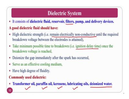
Dielectric System it consists of dielectric fluid, reservoir, filters, pumps and delivery devices normally you require filters because the debris will be a big problem if you do not have filters that the debris will re circulated the process. A good dielectric fluid should have the following properties, it should have high dielectric strength; that means, that remain electrically non-conductive until the required breakdown voltage is applied across the electrodes ok.
