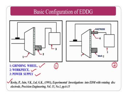
If you see the basic configuration of electric discharge diamond grinding process, you can directly you if you see 1 and 1 2 1 3 specifies the grinding wheel workpiece and power supply. So, normally you can supply directly to the workpiece itself and the grinding wheel are you can also give to certain electrode and you can go for the workpiece.
