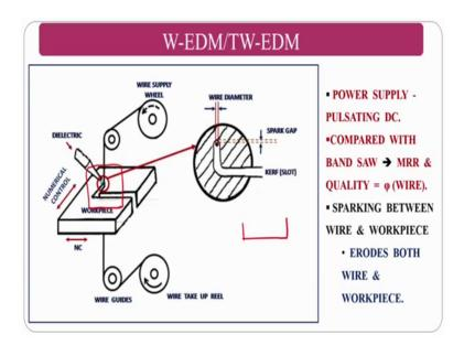
The material removal will action will be taken care by the electric discharge machining process mechanism only, here what will happen there will be a wire which is a conducting material workpiece also a conducting material wire is negative terminal as well as the workpiece is positive terminal and the dielectric fluid is fed here if you see here the dielectric fluid is fed. So, the mechanism of material removal will be same.
