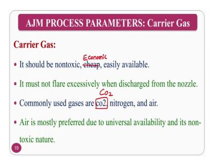
So, the second one is a carrier gas, normally carrier gas it should be non toxic, cheap, easily available. I can say instead of cheap you can say economic is a good word to use rather than cheap. It must not flare excessively when the discharge from the nozzle; that means, that it should not diverge much. If it is diverge then what is my requirement will be gone.
