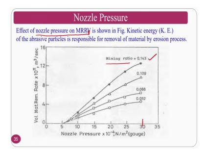
So, nozzle pressures, nozzle pressures with the volumetric material removal rate here you can see all the values. So, previous slide similar slide we have seen, but the thing is that there it is a qualitative one. As you increase it will increase, but how much increase of the input parameter will increase the how much output response that we are going to see here. Here 0.143 mixing ratio gives the highest value; that means, that mixing ratio is high.
