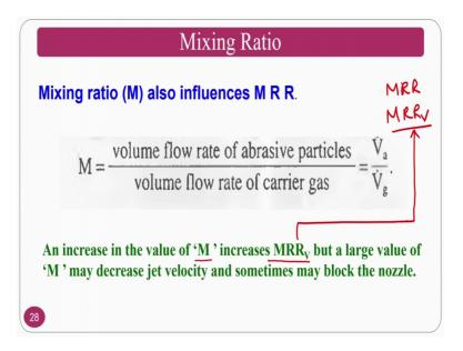
Just the mixing ratio so, the other keyword here is the mixing ratio that is nothing, but the volume flow rate of the abrasive particles to the volume flow rate of the carrier gas; that means, that you have 2 things here, one is a gas another one is a abrasive particles. If the mixing ratio is very high; that means, that your abrasives are higher in number compared to your carrier gas ok.
