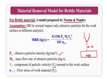
Material removal model for the brittle materials which is proposed by Neema and Pandey [FL], Professor Pandey; so, assumption material removal by normal impact only; that means, that there is no additional things involved. So, abrasive particles hit the work piece and the work piece material will be removed that is a simple assumption.
