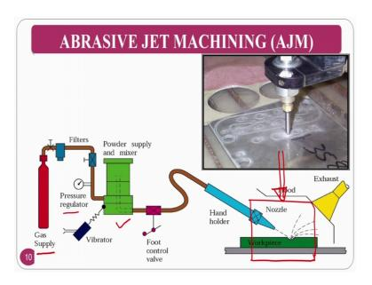
If you see the schematic diagram and the picture normally you can compress the gas supply normally air will be supplied. At the main motto to show you is how the system look like and you can also see the practical setups that are developed by some of the IIT's also. So, the gas supply filters are required to filter out the moisture or filter out the other things and which is unwanted and the pressure regulator just you mix the powders here and you can even give the vibrations to it.
