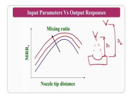
So, if you see the other parameters normally nozzle tip distance, if the nozzle tip distance is increases what is happens here is the crater diameters will. If the nozzle tip distance is low what will happen? The material removal will be good.
