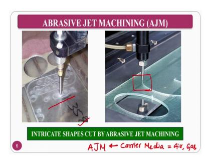
So, now based on this particular principle the people came up with a technology called abrasive jet machining. You can see the abrasive jet machining normally these are the highly compressed air along with the abrasive particles with impinge are which pass through a fine nozzle. And you can achieve or you can cut the intricate shapes like completes surfaces you can do and you can do a glass cutting or another cutting processes.
