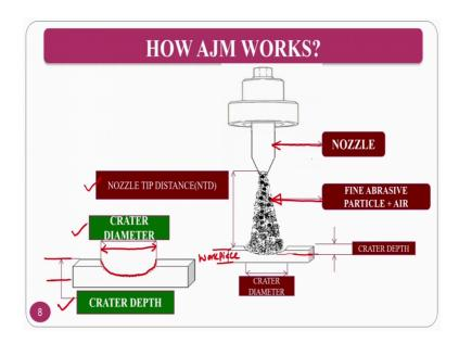
If you see here how the abrasive jet machining works, this is the nozzle ok. So, this is the nozzle tip distance, this is my work piece which is nothing, but the distance between work piece top surface to the nozzle exit is nothing, but nozzle tip distance. And fine abrasive particles plus air is coming here and this is the crater depth that normally this is a crater depth that is formed on a surface.
