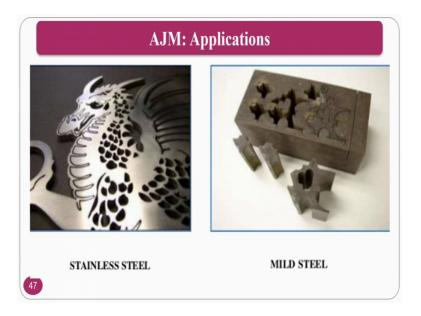
Stainless steel work pieces, you can see the good and complex structures are fabricated. At the same time thin structures and mild steel also can be cut. You see the thickness of this particular material, it is too thick material and you can cut using abrasive jet machining for this particular material, if some of the people might have used for by abrasive water jet machining also.
