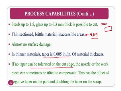
So, process capabilities still there are some more process capabilities, steels up to 1.5, glass up to 6.3mm thickness you can cut; that means, that if at all you have a steel plate of very small thickness, you can cut or your glass plates with big thickness you can cut using the abrasive jet machining. Thin sectioned, brittle materials, inaccessible areas can be machined by this particular AJM process.
