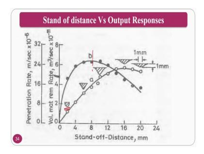
If you see the standoff distance with respect to volumetric material removal rate and the penetration rate is the penetration rate. If the standoff distance is too low, the normally the penetration rate is also somewhat low. But, if your penetration rate will be slightly increased if you give sufficient space are to the nozzle. If you give sufficient space to the nozzle what will happen? It has certain distance where it can carry the velocity and hit the work piece.
