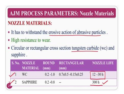
The nozzle material is most important one. So, it has to be it has to withstand the erosive action of abrasive particles that are passing by the nozzle. Because, the abrasive particles
