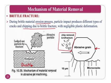
So, material removal mechanism, normally whatever you have seen in the previous slide that is for ductile material. If you are going for brittle material what will happen? During the brittle material erosion process, at the particle impact produces different types of cracks and the chipping is due to brittle fracture and negligible plastic deformation ok.
