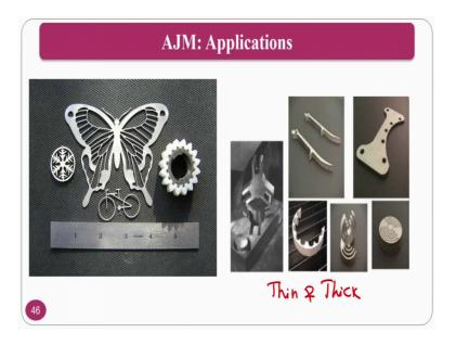
So, some of the applications as you can see the butterflies, dendrites structures, cycle structures and gears can be manufactured; at the same time many complex shapes with the thin structures and as well as thick structures can be made ok. Thin as well as thick structures one can cut using the abrasive jet machining process.
