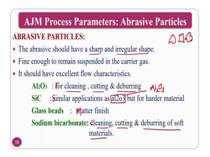
So, the first one is abrasive particles that play a major role. The abrasive should have the sharp and irregular shape. Normally, all the abrasive particles are randomly oriented at the same shape is random. One abrasive particle may like this; one abrasive particle may
