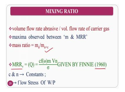
So, volumetric flow rate of abrasive to volumetric flow rates of carrier gas is nothing, but the mixing ratio. Normally, mass ratio also is there that is nothing, but mass of the abrasive particles to combination of mass of abrasive particle with carrier gas. So, volumetric material removal rate if you see here c f theta m V n which is given by the Finnie in 1960 where c and n are constant and the flow stress of the work piece is also given here.
