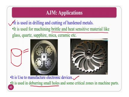
It is used to drill and cut the hardened metals normally you can do the drilling or cutting of the hardened metals also can be possible. It is used for machining of brittle and heat sensitive materials like glass, quartz, sapphire, mica, and ceramic. These are the some of the advanced materials where you can generate where you can make without any heat generation.
