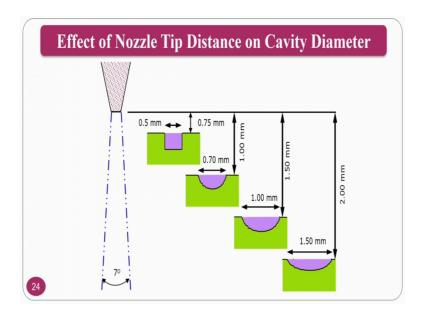
So, nozzle tip distance versus cavity, if the tip distance increases what will happen? The cavity diameter will increase and the depth will decrease. If you see here this is a schematic for your better understanding.
