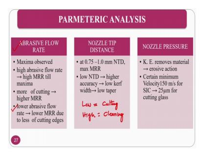
So, the parametric analysis if you see abrasive flow rate, the maximum observed normally high abrasive flow rate will lead to high material removal rate. The more cutting higher MRR, if the abrasive particle size is very big the cutting action will be very high and material removal will be very high. And low abrasive flow rate normally what will happen? To lower MRR due to less cutting edges and other things nozzle tip distance as I said.
