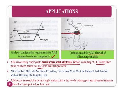
Applications, if you see the applications normally silicon or tungsten carbide configuration requirement for AJM for the trimming of electronic components. At the same time you can use AJM trimmed for the silicon you can use at different angles ok. You can use at different angles for trimming application this is one of the technique that you can use. AJM is successfully employed for manufacturing of small electronic devices consisting of 0.38mm thickness.
