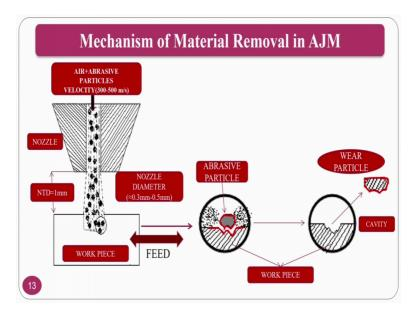
Mechanism of material removal if you seen the abrasives and nozzle tip distance and other things when the abrasive particle heat what will happen? It will fracture the material and the fracture mechanism and other things you will see in the upcoming slides.
