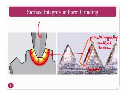
So, keep in mind whenever you report a research paper, the surface integrity in the form grinding basically if you see the form grinding like assume that we are going to do the Gears cutting and other things. What is going to happen here is if you see the surface here, normally a this is the parental surface and this is Metallurgically changed surface, Modified Surface ok.
