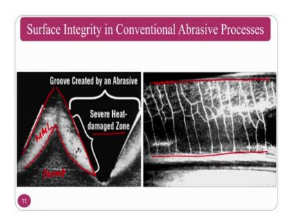
You can see, the group created by an Abrasive because of this you can you have seen the previous slides, where a structures are formed like grain structures are formed severe heat damaged zone is there and you can see, the metallurgically changed layer here ok. This is the parent material and this is a metallurgically modified layer.
