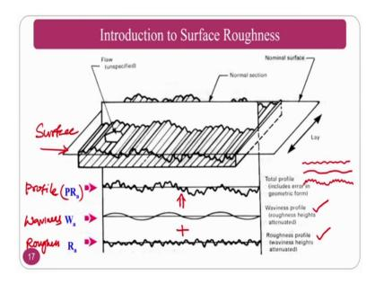
If you see this particular surface, the surface rough will have 3 things. This is the surface ok. So, the surface will have profile. This is called a Profile and PR a represents profile roughness. This is called Waviness and this is called Roughness ok. Waviness profile and roughness profile; if you club the roughness profile and waviness profiles, you are going to get the profile roughness.
