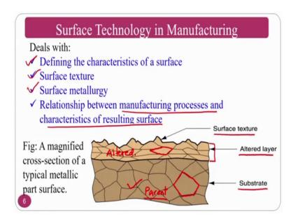
So, that means that the surface integrity has to be taken care that means, that not only you have to see the surface roughness, you have to see the metallurgical aspects also. This surface technology or the surface integrity defines the normally defines the characteristics of the surface, the Surface texture, Surface metallurgy and the relationship between the manufacturing process and the characteristics of resulting surface ok.
