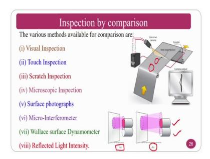
And the various methods available for comparison or like a Vision Inspection; that means, that you can visually see or the experience people see visually and they will compare with a master. Assume that I have a milling master and that the surface produced by a milling and the surfaces are that is to be supplied to the customer just you can compared by Visual Inspection method.
