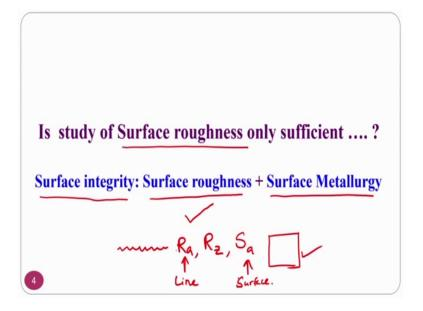
Is the Surface Roughness only sufficient? It is the question because if you see the previous slide, where the surface grinder is grinding the picture, where the lot of spark is generated ok. For that purpose, you always look at the Surface integrity that is nothing but the Surface Roughness plus Surface Metallurgy. These are the two things that one has to take care. But as an a mechanical engineer, we deal mostly with the surface roughness like R a.
