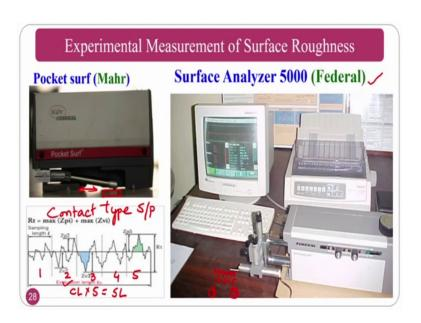
The Experimental method if you see as this is already saw by you in the previous slides. Again to understand for better understanding; for better understanding, I am showing again. If you can see the Pocket Surf and this is the Taylor surface analyser 5000. This is some made by the Federal. These are all we measure by the contact type. These are all contact type: surface profilometers.
