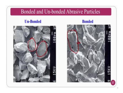
What is the difference between bonded abrasives and unbonded abrasives? If you see here the abrasive particles are individual entities, this is called unbonded abrasives as I said in the earlier slides also these are called bonded abrasives. You can see the periphery of the abrasive particles, it is completely bonded with a bonding material.
