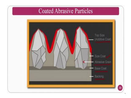
There are varieties of abrasive particles and some of the applications required coated abrasive particles ok. So, people also use as a coated abrasive particles now normally you can see the abrasive, additive coating is there at the same time size coating is there abrasive grain particle, you can see this is the abrasive grain and the base coating is done and backing material.
