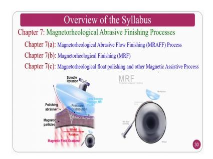
Whatever you are seeing here is MRF that is called magnetorheological finishing process, where you can also see the video how the magnetorheological finishing process
