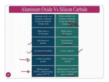
So, normally 2 abrasive particles are used in most of the machining and finishing applications that is called alumina or aluminium oxide and another one is silicon carbide. If you see the difference between these 2 particles, aluminium oxide or alumina is inorganic compound which a chemical formula A 1 2 O 3 and normally this is called as SiC silicon carbide ok.
