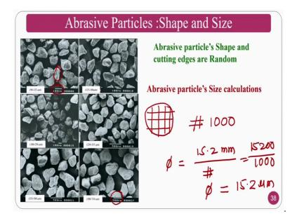
Shape and size normally you can see the size from course to fine to super fine, normally abrasive particles are divided into 4 segments course medium fine super fine ok. So, if you see here these are the course particles and whenever it comes to a big size, then it
