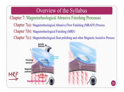
In this chapter 7 you will study about magnetorheological fluids where it is slurry basically. So, these fluids are used for sophisticated applications like contact lens polishing and other things. So, magnetorheological abrasive flow finishing process magnetorheological finishing process magnetorheological float polishing and magnetic assistive other process we will see.
