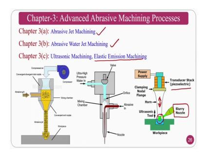
Coming to the advanced abrasive machining processes as you know, you are going to study about abrasive jet machining where abrasives are getting assistants from a compressed air, because the air is a carrier medium here and a abrasive particles will follow the path of injecting the air, but the air has a drawback that is it can diverge easily because of which the dimension that I want to get may be disrupted.
