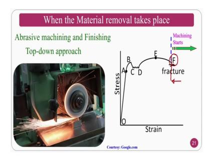
So, when the material removal takes place normally if you see the abrasive machining process, which is a top down approach in a grinding process or in a late process and other processes. Normally the machining takes place after the yielding bind; that means that, that is why these machining processes are called as severe plastic deformation processes ok. So, once the after this one only the material start sharing from the work piece ok.
