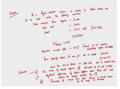
So, a problem in a hydroelectric scheme a number of Pelton wheels are to be used are to be used under the following condition right. Total output power required is equal to 30-megawatt gross head is equal to 245 metre, speed is equal to 39.27 radian per second, that is 6.25 revolution per second. It is given 2 jets per wheel Cv of the nozzle is equal to 0.97, that is coefficient of velocity.
