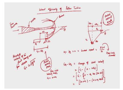
So, today we will discuss about wheel efficiency of a Pelton wheel Pelton of Pelton turbine. So, we need to draw the velocity triangles at the inlet and outlet so you know the bucket shape. So, suppose liquid is coming from the nozzle liquid from reservoir it is coming through the penstock, then it is taken to the nozzle. So, this is penstock, so this is from penstock, then this is nozzle and then the z is striking the buckets.
