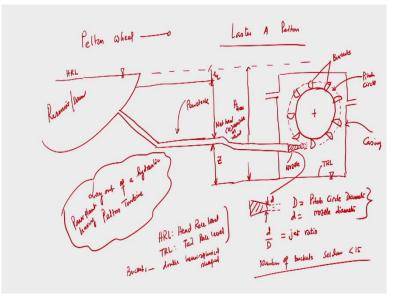
But the net head available on the wheel is H gross minus this height z and the frictional losses that is there when liquid fluid is flowing though the penstock.
