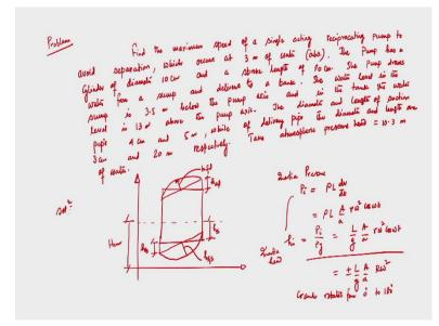
Now, if I go to the next slide and if I write the problem; so, problem is like this, find the maximum speed of a single acting reciprocating pump to avoid separation to avoid separation which occurs at 3 meter of water, which occurs at 3 meter of water this is absolute. The pump has a single of diameter the pump has a cylinder has a cylinder of diameter 10 centimeter and a stroke length of 20 centimeter a stroke length of 20 centimeter.
