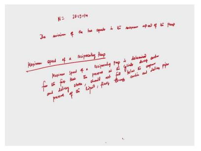
So, value of N will be that you know 28.59 rpm. So, maximum speed during delivery stroke without separation is obtained is the 28.59 operation. So now, the question is find the maximum speed of a single act reciprocating pump about separation which occurs? So, the minimum of these two speeds is the maximum speed of the pump, now question is the minimum of the two speeds is the maximum speed of the pump, two avoid separation and so, that it is given.
