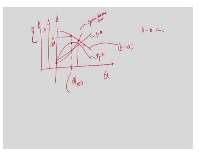
Now, we will discuss about the one you know pump characteristic curve that I have discussed that pump characteristics curve are H Q curve. We have seen that you know pump should have if I plot the experimental data; if I plot the experimental data; I will get I will get the pump H Q curve like this.
