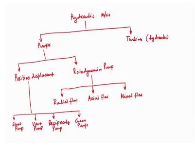
So, hydraulic machines, hydraulic machines one is as I said that there be again positive displacement pump, it may be a positive displacement pump or I can say that there may be pumps, hydraulic machines pumps or we have a turbine, hydraulic turbine.
