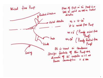
So, this is again pump axis, this is blade, this is bud, this is pump casings. Now, here, the blade or the hub makes an angle alpha with the axis of the machine. So, this is angle alpha.
