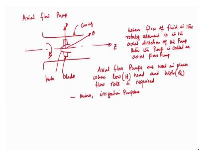
Next, we will go for the axial flow pump, axial flow pump. So, again I will draw schematic. So, this is hub plus blades which is known as imp impeller. So, these are pump casings, this is casing, which surrounds the impeller, this is known as blade and this is hub, so, hub plus blades which is impeller, which is surrounded by a casing. Now, we have a three directions Z, R and  $\theta$ .
