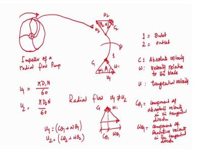
So, if I draw impeller that is hub as well as blade of and suppose, pump is impeller is rotating in the clockwise direction.
