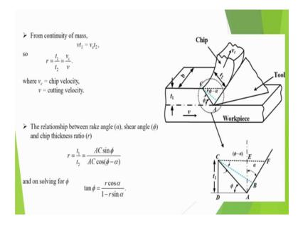
From the continuity of mass v t 1 is equal to v c t 2 that also we can do in the width direction the chip is not spreading. So, we get v t 1 is equal to v c t 2 like that. And then r is equal to that is cutting ratios t 1 by t 2. So, cutting ratio is basically nothing but v v c by v, v c is the chip velocity and v is the cutting velocity at most the cutting velocity can be equal to 1. So, v c can at most be equal to v.
