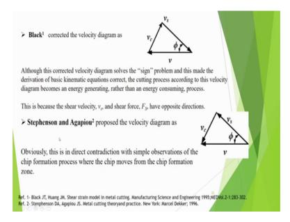
So, Black, corrected the diagram like this Black as need this type of diagram blacks peoples also there although this corrective velocity diagrams are the sign problem. But in this diagram also there is a some problem because shear force and v s both are in opposite direction, then there are some other authors they propose another type of velocity diagram.
