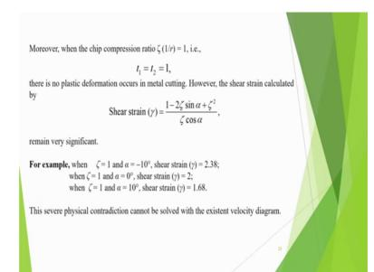
Moreover when the chip compression ratio is one suppose chip compression ratio is one that is t 1 is equal to t 2 actually there should not be any plastic deformation in metal cutting it is just rotation type of thing. But you are calculating the shear strain using this formula then you will still be getting some shear strain because this formula is 1 minus 2 tau sine alpha plus tau square by tau cos alpha. So, put tau sorry it is it should be called zeta and this is what zeta is this one.
