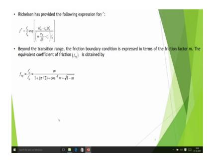
T s star time being expressed in this manner, f star is equal to this one; f star basically so that means, the if we are in this region then the Coulomb's coefficient of friction equivalent Coulomb's coefficient of friction is in fact, dependent on what is the amount of the normal stress T n. So that is what by this expression is dependent like this it is a function of t n.
