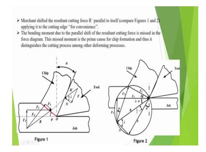
Merchant shifted the resultant cutting force R prime parallel to itself just see if you compare the figure that here he is making that actually the forces are acting here, but in the merchant circuit diagram they are shown here in this one at the tool point is considering this as tool tip.
