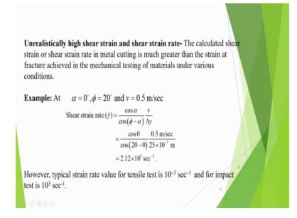
And then unrealistically high shear strain and shear strain rates are predicted by this model Astakhov feels that the strain rate may not be actually that high it may be only of the order of 10 per second. But these flow (Refer Time: 44:03) predict 10 to the power 5 etcetera. Calculated shear strain are shear strain rate in metal cutting is much greater than these strain at fracture achieved in the mechanical testing of materials under various conditions. I give one example.
