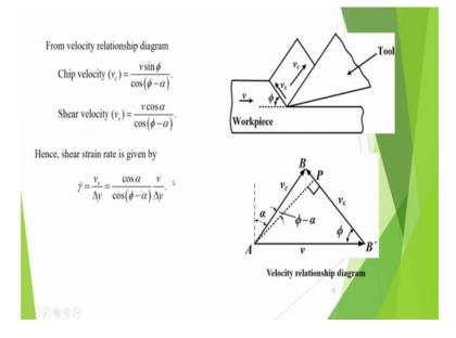
Now, from the velocity relationship diagram suppose we go to the velocity relationship that suppose it is v and then there is a chip is moving here chip may be sliding up. So, v s is shown up job is moving with velocity v and this is v c, v c is the chip velocity we call chip velocity we can make it triangle. Triangle because these are vectors, so suppose v is the workpiece on which there is a chip which is sliding with v s.
