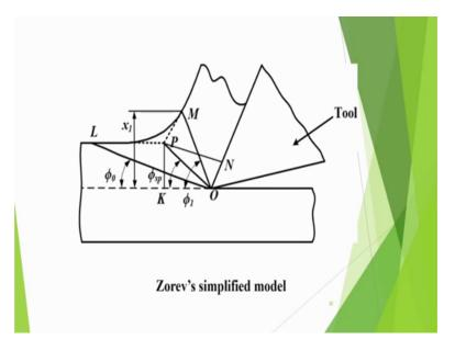
He simplified this ultimately again and he said let this curve portion should be taken as a straight line, then he is getting this type of model here and this and this may be that he has taken some representative value of this one, that shear angle ultimately it boils down to single shear plane model and this one.
