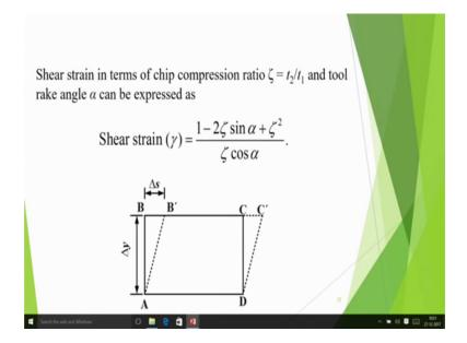
Now, here shear strain can also be expressed in terms of the chip compression ratio. I defined the cutting ratio cutting ratio is t 1 by t 2 chip compression ratio is exactly reverse of that. So, this is the find as t 2 by t 1. Cutting ratio is always less than 1, chip compression ratio is actually more than 1 and shear strain can be expressed as a function of chip compression ratio and rake angle alpha because phi is also dependent on chip compression ratio and rake angle.
