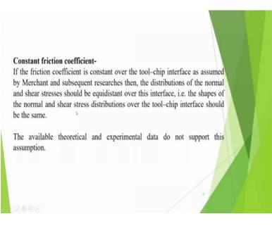
And naturally the constant friction coefficient has been taken if the friction coefficient is constant over the tool chip interface as assumed by Merchant and subsequently researchers. Then the distribution of the normal and shear stress should be equidistant over this interface that is the shapes of the normal and shear stress distribution over the tool chip interface should be the same, but that is not true. I already have shown that how these shapes look.
