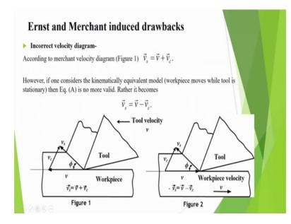
And then Astakhov pointed out that Ernst and Merchant including some drawbacks in the velocity diagram because merchant model the velocity diagram like this. In this case he assumed that the tool is moving with velocity v and in that case v s is equal to v plus v s, but if we take the equivalent model in that case this minus v s will be equal to v minus v s.
