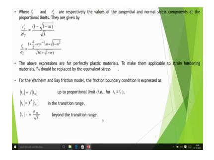
These expressions are for perfectly plastic material that means, we assume that the material means rigid and after certain point it becomes a plastic all of a sudden that is rigid and there is no strain hardening. So, to make them applicable to strain hardening material sigma eq in these equations can be replaced by the equivalent stress that means, sigma Y also I can use that other expression which is dependent on the strain hardening similarly sigma Y may be dependent on the temperature also.
