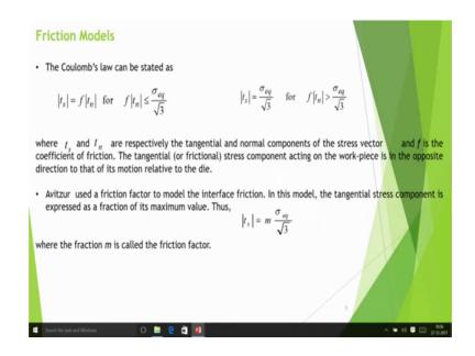
Here, so Coulomb's model can be stated as t s is equal to f times t n, where f is the coefficient of friction, but provided a f times t n that means, the total shear is stress is somewhat is smaller than sigma eq by root 3. What is sigma eq? That means, equivalent stress in terms that means, may be that I can write it sigma Y if I am not considering the temperature and strain effect, so sigma Y by root 3 that means, maximum shear yield stress.
