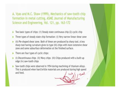
There is one good paper by Vyas and Shaw which was published in a ASME journal of Manufacturing Science and Engineering in 19 9 1999, volume 121. It is about 10 page paper in which he has classified the chips into two types, one is steady state continuous chip like this and other is basically the cyclic chips.
