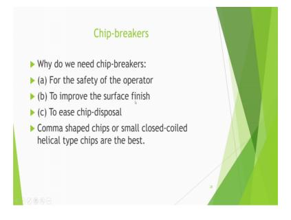
Why we need to break the chips? It is because of the for the safety of the operators to improve the surface finish and to ease chip disposal. These are the three main important things. The safety of operator because operators and it can come then improve the
