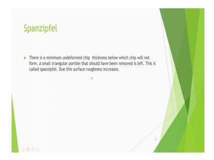
Here one thing I have not shown, but we can also get sometimes this type of effect that actually formation of a chip, you need minimum undeformed chip thickness minimum uncut chip thickness. If that is not there then chip will not form instead a small triangular portion that should have n been removed is left and this is called the spanzipfel due to this surface roughness increases.
