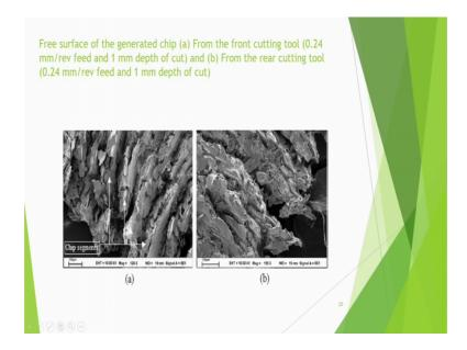
And, then three surface of the generated chip is also shown here, he is finding some segments here. These are the chip segments; that means, they are cutting he also this is this one he observed in both the cases.
