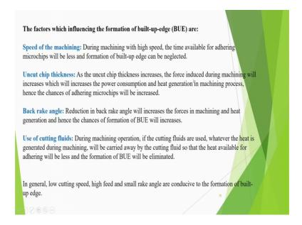
The factors which influence the formation of built-up-edge are speed of the machining that is important. During machining with high speed the time available for adhering microchips will be less and formation of built-up-edge can be neglected. So, formation of built-up-edge can be neglected that is why that is a speed helps in eliminating built-up-edge.
