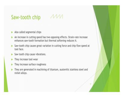
So, saw tooth chip like this one typically a schematic diagram, I have shown here they are also called segmental chips and increase in cutting speed has generally two opposing effect strain rate increases enhances saw tooth formation. Because as you know the strain rate increase we will have tendency to increase the flow stress of the material, more difficulty in cutting, but the thermal softening has opposite effect; it reduces it.
