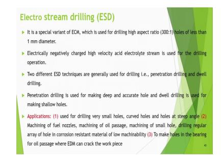
A variant of this process is electro stream drilling. It is a special type of ECM which is used for drilling of high aspect ratio 300 to 1 holes of less than 1 mm diameter. So, aspect ratio can be that much high; that means, length of the hole can be 300 time than its diameter.
