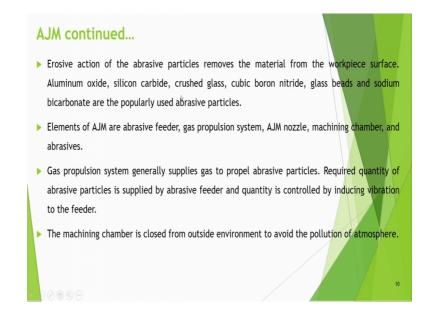
Now erosive action of the abrasive particles removes the material from the workpiece surface aluminum oxide, silicon carbide, crushed glass, cubic boron, nitride glass beads and sodium bicarbonate are the popularly used abrasive particles. So, these are the abrasive particles. Elements of AJM are abrasive feeder gas propulsion system AJM nozzle machining chamber and abrasives.
