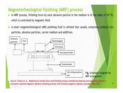
Now, magneto rheological finishing process in MRF process, finishing force by each abrasive particle in the medium is of the order of 10 to the power minus 9 Newton. So, magneto rheological finishing process will use some magnetorhelogical medium which will change its viscosity depending on the magnetic field. So, forces are of very small
