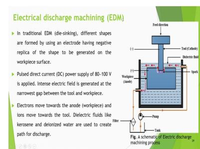
Example is electrical discharge machining in traditional EDM that is called die sinking because it makes a die type of thing different shapes are form by using an electrode having negative replica of the shape to be generated on the workpiece.
