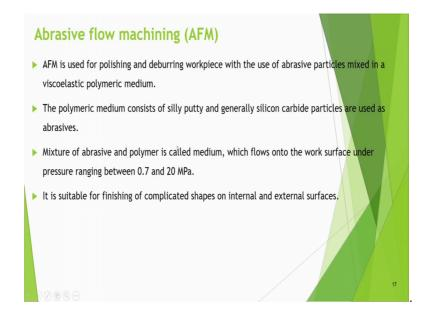
Now I am only discussing about the mechanical processes in which mechanical energy is there; that means, there is a physical contact between the medium and the workpiece. So, abrasive flow machining process is another type of such type of process. In abrasive flow machining we do polishing and deburring of workpiece with the use of abrasive particles mixed in a viscoelastic polymeric medium we can usually call it a putty.
