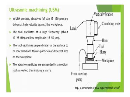
Here ultrasonic machining. Now, just see the diagram of ultrasonic machining I am imparting vertical ultrasonic vibrations. These are the leads, then I am circulating the water. Then this is a that horn the purpose is to implify the vibrations, then I have got a
