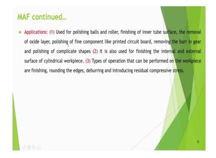
It is also used for finishing the internal and external surfaces of cylindrical workpiece. Types of operation that can be performed on the workpiece are finishing, rounding the edges, deburring and introducing residual compressive stresses.
