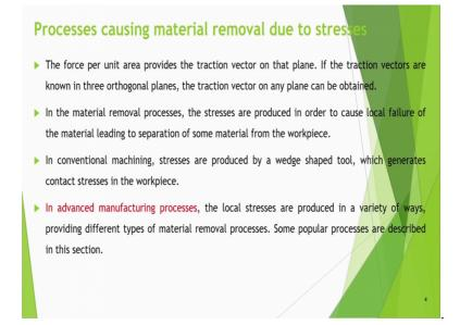
Let us discuss mechanical types of processes; that means mechanical processes or I would better name them as processes causing material removal due to stresses. That
