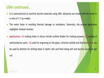
So, this I have shown, now it is uneconomical to machine ductile materials using USM abrasives are mixed with the water in a ratio of 1 isto 1 by weight. So, that is what suppose you may have 1 kg of a abrasive and 1 kg of water and you can make a slurry.
