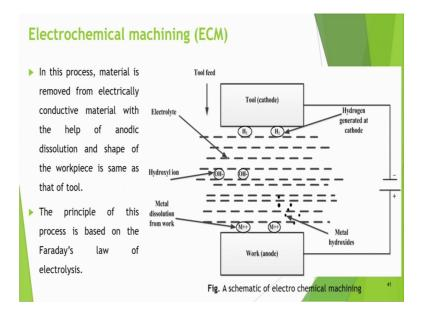
Now, I am going to discuss about electrochemical machining. So, this is quite different from the previous processes here it works on the Faraday's law of electrochemistry. Suppose workpiece is anode and tool is of cathode connected to negative one and this is
