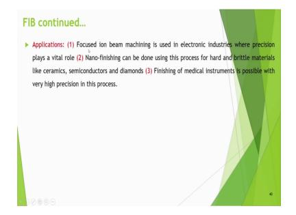
So, applications can be focused ion beam machining is used in electronic industries where precision plays vital role. Nano-finishing can be done using this process for hard and brittle materials like ceramics semiconductors and diamonds. Then finishing of medical instruments is possible with very high precision in this process.
