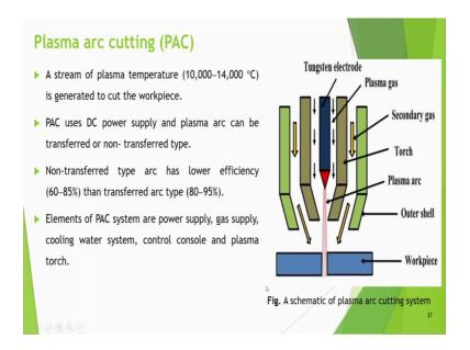
And plasma arc machining, it is also similar to laser beam machining, but here we are using a plasma. Suppose we have a tungsten electrode and which can be provided with the DC supply. A stream of plasma is basically ionized form of the gas in which there are ion. So, a stream of plasma temperature that is 10000 to 14000 degree generated to cut the workpiece. Plasma arc used DC power supply and plasma arc can be transferred or non transferred.
