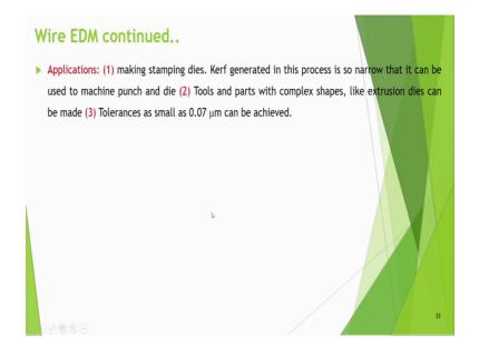
So, applications are making stamping dies. Kerf are cut generated in this process is narrow that it can be used to machine punch and die. Tools and parts with complex shapes, like extrusion die can be made. Tolerances as small as 0.07 micrometer can be achieved.
