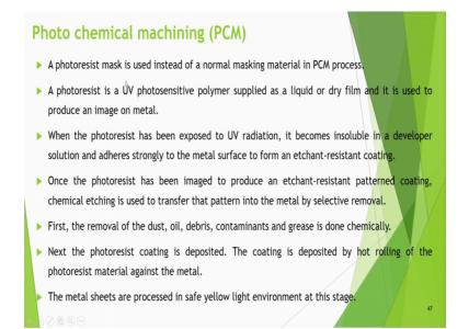
Then photo chemical machining is like a chemical machining only, but here a photoresist mask is used instead of a normal masking material in chemical machining process. A photoresist is a ultraviolet photosensitive polymer supplied as a liquid or dry film and it is used to produce on image on metal. When the photoresist has been exposed to ultraviolet radiation, it becomes insoluble in a developer solution and adheres strongly to the metal surface to form an etchant resistant coating.
