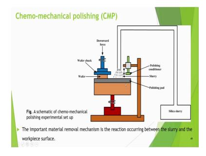
Then this is chemical mechanical polishing. This is basically chemical as well as mechanical action is there. This is shown that silica slurry is there, it is coming through this. This is a polishing conditioner and this is a polishing pad this is some wafer which you are going to machine.
