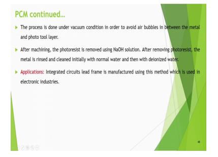
The process is done under vacuum condition in order to avoid air bubbles in between the metal and photo tool layer. After machining the photoresist is removed using NaOH solution. After removing photoresist the metal is rinsed and cleaned initially with normal water and then with deionized water. Applications include integrated circuits lead frame is manufactured using this method which is used in electronic industry.
