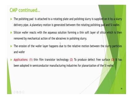
So, this is a wafer chuck and you are machining that wafer. So, in this important material, removal mechanism is the reaction occurring between this slurry and the workpiece surface. And the polishing pad is attached to a rotating plate like this, this is
