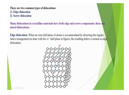
And here there are two common types of dislocations one is called edge dislocation other is called screw dislocation. Many dislocations in crystalline materials have both edge and screw components these are mixed dislocations.
