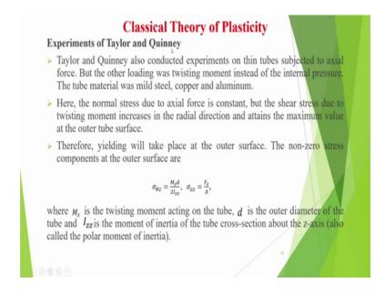
Now, then similarly experiments of Taylor and Quinney they conducted the experiments on this tubes, but subjected to axial force, but instead of applying any pressure they applied the twisting moment.
