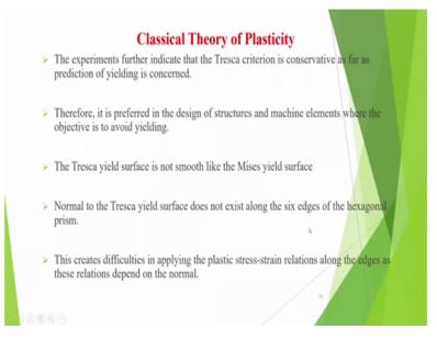
So, the experiments indicate that the Tresca criteria is conservative as for as the prediction of yielding is concern that means, according to Tresca criteria yielding will start first.
