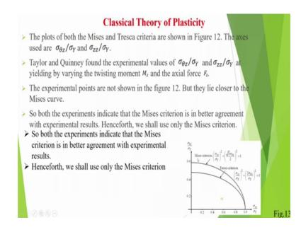
So, both the criteria are here plotted nicely in this expression, this is Mises criteria this is Tresca criteria. So, most of the experimental points they lie between these two criteria, so we can see, but Mises criteria predicts more stresses compare to the Tresca criteria.
