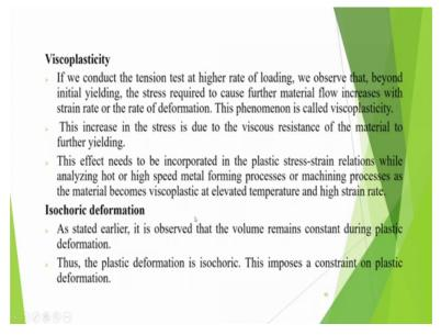
So now, we discuss that what is viceoplasticity? If we conduct the tension test at higher rate of loading we observe that beyond initial yielding the stress required to cause further material flow increases with strain rate or the rate of deformation. That means it is dependent on the rate of deformation. If you conduct the test at slow strain rate you will have different observation, if you conduct the same test at high strain rate you will have different observation.
