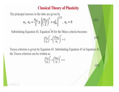
And then the principal stresses in the tube are given by sigma 1 sigma 3 and sigma 2 equal to 0, then the one Mises criteria becomes like this and the Tresca become like this.
