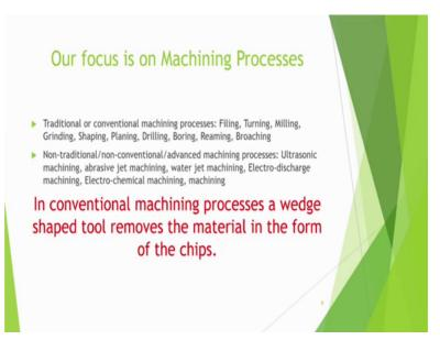
So, first we discuss conventional machining process. In conventional machining process a wedge shape tool removes the material in the form of the chips and we also analyzed that why do we use a wedge shaped tool because it acts as an incline application device. We apply some force, but the normal force is amplified.
