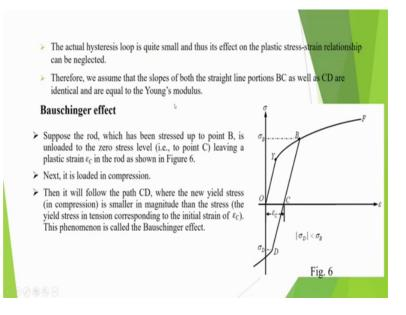
So, actual hysteresis loop is quite small and thus its effect on the plastic stress strain relationship can be neglected therefore, we assume that this slopes of both the straight line portion BC as well as CD are identical and they are equal to Young's modulus. I told that unloading is also elastic. Now, we are going to discuss another effect that is called Bauschinger effect.
