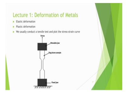
One common test is the uniaxial tensile test in which we make a dog bone sample and we fix it between one movable jaw and one fixed jaw and then after that we apply the force.
