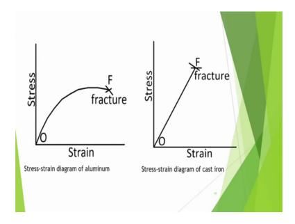
And now coming to the next one we told that stress strain diagram for aluminum, stress strain diagram for cast iron which is a brittle material. We told that definition of nominal stress and true stress and we also told that how they are related.
