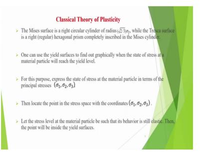
So, now, you all observing like this here. So, Mises surface is basically a right circular cylinder of radius under root 2 by 3 sigma Y; while the Tresca surface is a right regular hexagonal prism completely inscribed in the Mises cylinder. So, Tresca remains inside the one Mises that means Tresca is conservative, that means if the material is failing as per one Mises it will definitely fail as per Tresca.
