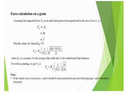
Now, about coming about force calculation on a typical grain, assuming that the tangential force F g on an individual grain to be proportional to the area of cut A c that is suppose F g is proportional to A c. And area of cut can be taken proportional to width of this one and thickness t b t. And since b is roughly proportional to t; that means, width is more than naturally we can have assume that may be thickness is also more, I thickness is more than the width is more.
