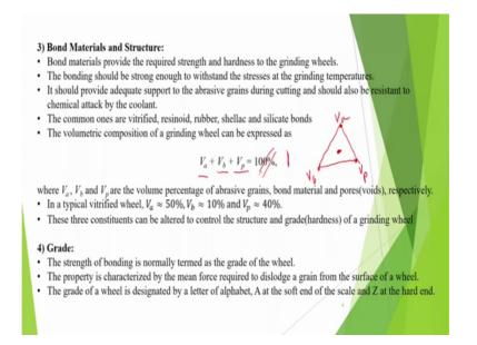
Bond materials provide the required strength and hardness to the grinding wheels, because abrasives are basically loose particles. So, they have to be bonded together. So, these abrasives are bond together. And the bonding should be strong enough to withstand the stresses at the grinding temperature. Because temperature also increases there is lot of heat generation. So, bonding should be strong, otherwise the abrasives will fragment and nothing will be done you cannot do machining.
