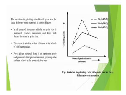
So, it is like this here. The variation in grinding ratio G with grain size also is shown increases initially with grain size, but reaches maximum and then with further increase in grain size, it reduces, it is similar to previous curve for a given material there is an optimum grade. And there is optimum grain size also. So, this has been shown here.
