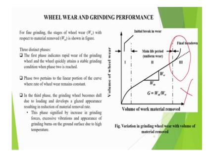
Now, wheel wear and grinding performance for fine grinding the stages of wheel wear W with respect to material removed W m is shown in figure. So, volume of wheel wear and volume of work material removed is plotted here. G is the grinding ratio that is volume of material removed divided by volume of the wheel remove thing removed, wheel material removed.
