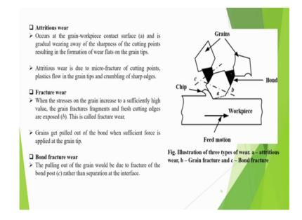
Now, what are the wears of the grinding wheel? That means, attritious wear we told that it is basically due to contact and rubbing. It occurs at the grain work piece contact surface, and is gradual wearing away of the sharpness of the cutting points, resulting in the formation of wear flats on the grain tips. Now attritious wear is due to micro fracture of cutting points. Plastics flow in grain tips, not plastics flow it is plastic flow and crumbling of sharp edges, sharp edges get crumbled.
