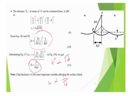
And then distance s f in terms of h can be evaluated from triangle ABC like here. And this is S f by 2 D by 2 square D by; So, s f is equal to under root 2 D h. So, equate both the portions h is this so, you get h is equal to this much. And substituting the expression for t we get h is equal to t square by 16 d. So, that means, basically this that peak to valley height h. That is proportional to t square, but it is 16 by d that means inversely.
