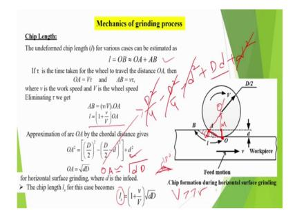
Now let us discuss about the mechanics of grinding process. You have to little bit visualise and put some effort. It uses lot of geometry and some trigonometry; that suppose consider a surface grinding type of operation. In which suppose work piece is moving like this and there is a wheel. Relative motion is only important suppose the table is reciprocating or moving in this direction, wheel may be stationary or alternatively the wheel can move and this can be this one.
