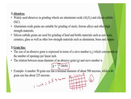
So, let us discuss one by one about abrasive abrasives widely used. Abrasives in grinding wheels are aluminium oxide, that we say Al 2 O 3 and silicon carbide that is SiC. Aluminium oxide grains are suitable for grinding of steels ferrous alloys and other high strength materials. Aluminium oxide grains are suitable; suppose, you want to grind steel you can use aluminium oxide ferrous alloys are there, and some high strength materials can be machined or ground by aluminium oxide.
