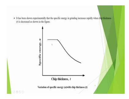
Now it has been shown experimentally that specific energy in grinding increases rapidly when chip thickness t is decreased. Like here, it is increasing very rapidly for high chip thickness it is less, but then it increases that we called so called size effect.
