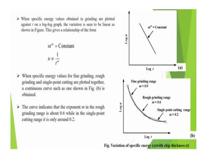
When a specific energy values obtained in grinding are plotted against t on log log graph, the variation is seen to be linear. This gives a relation in the form u t m is equal to constant or u is proportional to 1 by t m. So, when a specific energy values for fine grinding rough grinding and single point cutting are plotted together, a continuous curve
