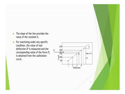
Now let us go to this one slope of the line provides the value of constant k for machining under any specific condition, the value of tool deflection delta star is measured. I have measured this delta star and the corresponding value of the force Pz is obtained from the
