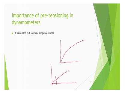
Now we have to we have to put some pre tension in dynamometers it is carried out to make response linear; that means, initially you have to apply some load suppose relation between the force and this one is like this, like this ok.
