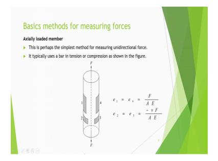
So, let us discuss first the measurement of the forces by means of the a strain gauges. Consider that there is axially loaded member, this is some member and in which some force as being applied on both sides. Now you want to measure this force. So, it is very simple method. In this is a bar, it will be it can be put in tension or compression.
