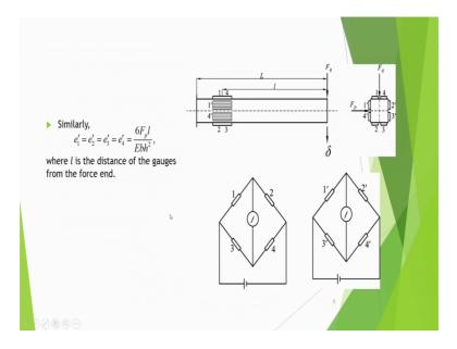
Similarly, e 1 prime e 2 prime e 3 prime e 4 prime is equal to 6 F p L divided by E b h square where L is the distance of the gauges from the forced end. So, that is what this has been done and these things have been arranged like this.
