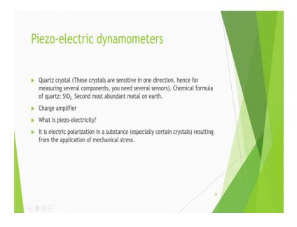
And then at quartz crystal these crystals are sensitive in one directions. Hence for measuring several components you need several sensors. Because it is if you want to measure horizontal force then it should be put in that direction.
