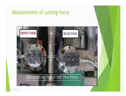
So, it is the we have actually measured in our workshop cutting forces. We have got the we are doing double tool turning one tool is here one tool is here. Now distance between the 2 tools is separated it is shown here. And we are putting this 2 dynamometers and they are connected by cables, that cable is going into charge amplifier and this one. So, this we are doing.
