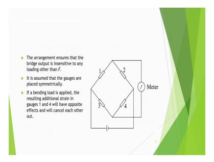
Now, here this arrangement this type of arrangement ensures that the bridge output is insensitive to any loading other than F. Suppose, there is a cross loading etcetera then that effect will be minimized. It is assumed that the gauges are placed symmetrically. If a
