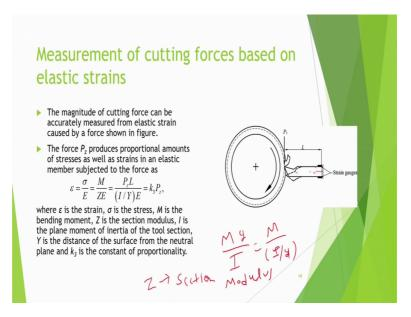
So, it is now the magnitude of magnitude of cutting force can be accurately measured from elastic strain caused by a force shown in figure; that means, I can instead of measuring the deflection now I can measure the strain shear.
