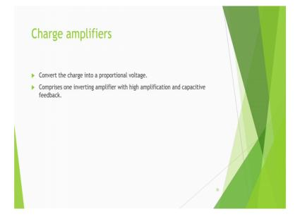
Charge amplifiers they convert the charge into a proportional voltage. And it comprises one inverting amplifier with high amplification and capacitive feedback. So, these type of things are do.
