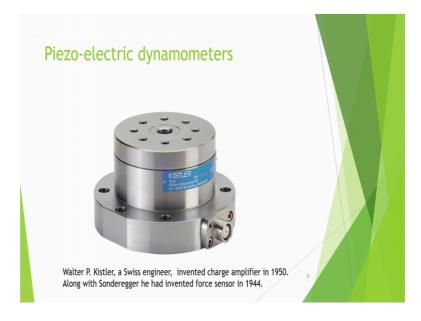
So, it is a typical that piezoelectric dynamometer is shown here. This I have taken photograph from my workshop. And this is a Walter P Kistler was one Swiss engineer who invented charge amplifier in 1950 by putting piezoelectric crystals. And a along with before that along with Sonderegger he had invented force sensor in 1944.
