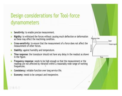
So, this we can measure. So, most of the dynamometers are produced and they are having this type of. Particularly crystal is making this dynamometer other companies also sometimes making this type of dynamometers. They are based on the piezoelectric crystals.
