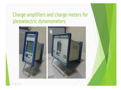
Now, this is these are basically called charge amplifier because, of the compression of the piezoelectric crystal charge is generated, but that may be small. So, you have to amplify it and then properly you have to measure also. So, complete amplifying and this one measurement is done by charge meter. So, these are charge amplifier and charge meters combined for Kistler dynamometers this we have taken.
