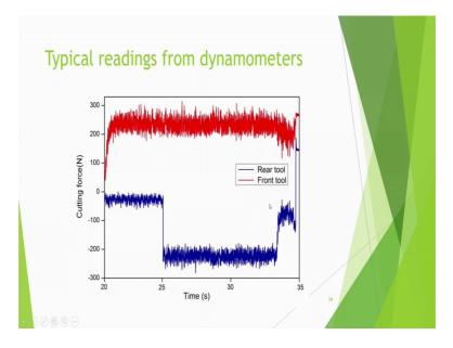
And then typical readings from dynamometers we are getting like this. See cutting force from the front tool it came like this. More than 200 and something just than 300
