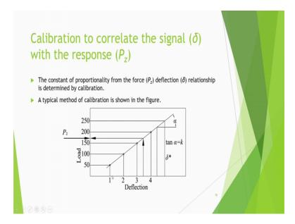
So, we see that delta and Pz both are proportional to each other and we can plot if we graphically, if we do calibration means first you have to calibrate we have to see that with known load we measure the deflection. We understand the instrument what is the relation between the force and deflection. So, that process is called calibration. After that you can use. So, we have to do calibration to correlate the signal delta with the response Pz.
