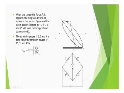
Now, when the tangential force F p is applied; suppose, you apply the tangential force F p then the ring will deform as shown in this second figure. And the strain gauges are located at 1 prime 2 prime 3 prime and 4 prime; that means, at these locations you will have you will make the bridge. So, these gauges will be there. Here 1 prime then 4 prime
