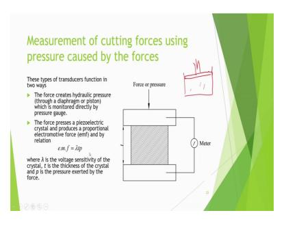
Strain now we can measure cutting forces using pressure caused by the forces also we can measure the pressure. So, these type of transducers function in 2 ways. One is force creates hydraulic pressure, we can put a hydraulic cylinder on top of this there will be piston. And if we put some suppose put a force here naturally this will produce pressure
