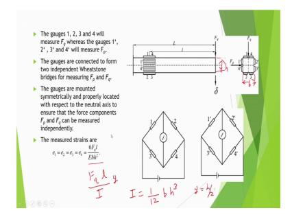
So, gauges 1, 2, 3 and 4 will measure F q, whereas, the gauges 1 prime, 2 prime, 3 prime and 4 prime will measure F p. So, here we have got total 8 gauges. Now, we put lie this; the gauges are connected to form 2 independent Wheatstone gauges for measuring F p and F q. So, we have arranged like this. This is one and 4 because they are having same type of strain. So, we have put on the opposite side. So, that effect gets amplified and this is 2 and 3 and in between I am measuring the voltage.
