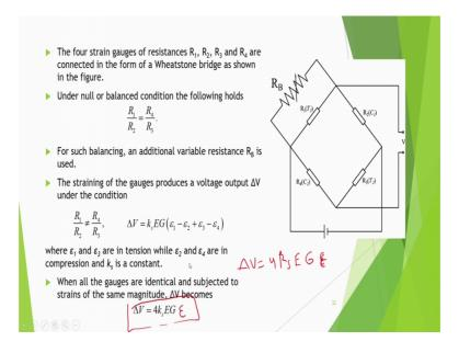
So, then the 4 strain gauges resistance R 1 R 2 R 3 and R 4 are connected to Wheatstone bridge. So, in this case may be if it is tension, then R one may increase R 3 may increase R 4 and R 2 may decrease. Under null or balanced condition the following thing will hold this you can even in your plus 2 level also you have studied, that about Wheatstone bridge that if there is a if it is totally balanced in that case R 1 by R 2 will be equal to R 4 by R 3.
