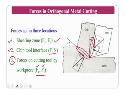
So, there are the forces in orthogonal metal cutting that is a machining processes; force act in three locations one is shearing zone if you see the shearing zone that is nothing, but the shear force and normal to the shear force; this is a shearing zone. So, the chip tool interface the other forces that one observes in this region is chip tool interface.
