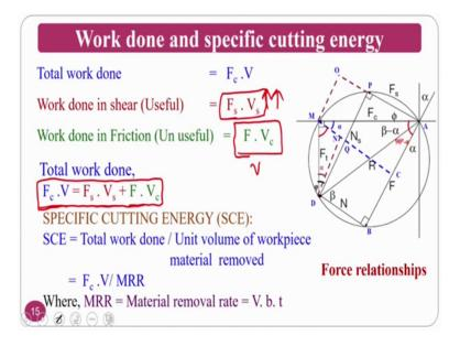
Work done in in specific cutting energy; so, now, work done total work done is F c into V. As I already said the cutting force multiplied by the cutting velocity is the total work that is done during the machining operation or that am imparting that is the energy.
