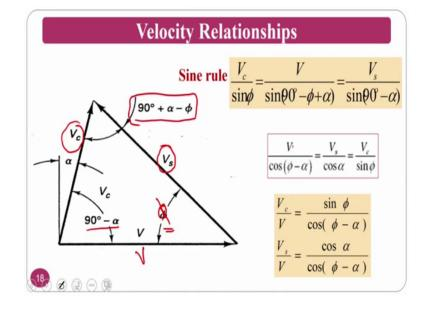
So, if you can see clearly for the for understanding purpose; this is the phi, this is 90 minus alpha, this is 90 plus, this phi minus alpha minus phi ok.
