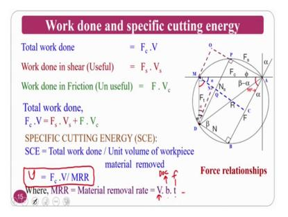
Specific cutting energy normally represent in terms of U basically. So, specific cutting energy is nothing, but energy given to the material removal rate ok; how much is removed per unit time volume that is nothing, but my chip thickness; that means, uncut thickness into the this is called my feed, this is called my depth of cut and this is called my cutting velocity.
