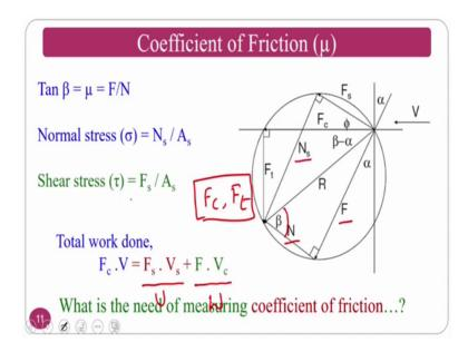
The coefficient of friction; the first thing what we are going to calculate from this one is the co efficient of friction. The co efficient of friction is nothing, but tan beta; so, this is my beta angle, tan beta equal to F by N that is mu this is coefficient of friction that I am going to calculate.
