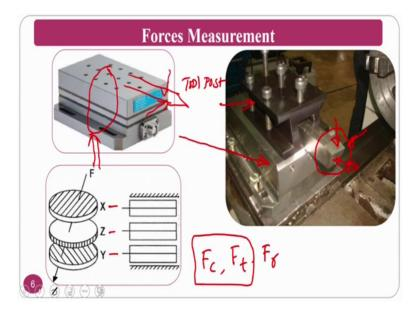
So, the force measurement if you see the force measurement normally this is the dynamometer you can see which is located beneath the tool. This is the tool this is a tool post, this is the tool post or the tool holder you can say this the dynamometer.
