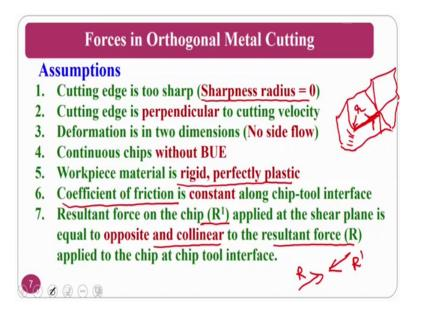
So, to have the Merchant circle relation; we are going to have some of the assumptions to measure this forces. This assumptions are cutting edge is too sharp; that means, that sharpness radius is 0.
