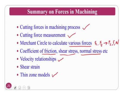
So, summary of this is what the cutting forces in the machining process is done. The cutting force measurement how using dynamometer and all those things and the Merchant circle to the calculate various forces.
