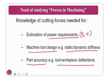
So first we should know what is the need of studying the forces in machining operation? If you see the knowledge of cutting forces is required to estimation of the power requirements. Normally power requirements, if you see it is F c into V; so, if you can calculate the cutting force and you know the velocity cutting velocity. So, you can calculate the what is the power required or the energy required.
