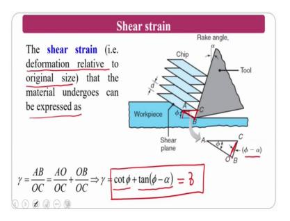
Now, we are going to calculate what is the shear strain; the shear strain that is the deformation related to the originals original size; so, that is the material undergoes as explained as possible that is nothing, but the gamma, so gamma is nothing, but AB by OC.
