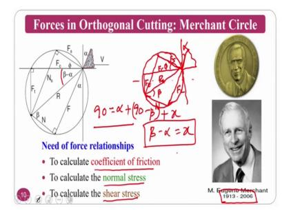
So, this is what you can see; so, now, you can see the same picture here the Merchant circle, where Merchant is the person invented it and all those things. The need for force relations to calculate the coefficient of friction the normal stress and the shear stress as I said in the previous one. So, I will let you know how to draw simply ok.
