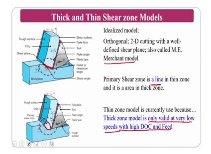
So, there are thin zone models and thick zone models. So, the thin and thick zone models; so, normally idealized model; the orthogonal 2 D cutting with the well defined shear plane also called as a Merchant model this is called thin zone model.
