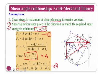
That is Ernst Merchant theory; so, the first assumption is shear stress is maximum at the shear plane and it remains constant that is nothing, but the shear stress is maximum and it is constant ok.
