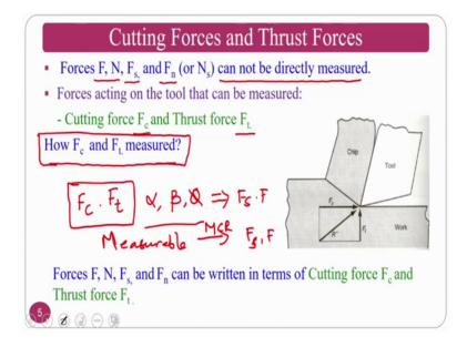
So, the forces F that is frictional force normal to the friction force shear force and normal to the shear force. These are all not calculated directly ok, these are all measure from a relation forced relation that is which we will see in the upcoming slides which is nothing, but the Merchant circular relation. The forces acting on the tool that is nothing, but the cutting force and thrust force also other forces if you have a dynamometer of which two components you can measure F c and F t.
