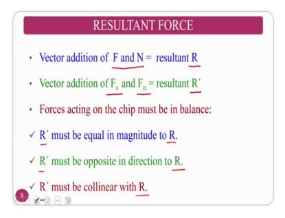
Vector addition of the frictional force normal to the frictional force resulting; in R that is the resultant force. So, vector addition of shear force normal to the shear force gives rest to the again R and the force act acting on the chip must be balance for that purpose R is equivalent to R; R must be in opposite direction to the R; so, R dash must be collinear with R. (Refer Slide Time: 17:38)
