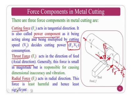
So, if you see there are three force components in the metal cutting operation; one is cutting force, second is the thrust force and the radial force; these are the three forces. The normally the cutting forces tangential to direction it is also called as a power component, normally this is as I said in a beginning of this forces F c into V gives me the power requirement.
