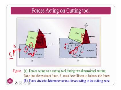
So, now we will move to the forces acting in the cutting tool since we have already seen in the previous to previous slide. So, there the forces if you see this is the shear and this is the normal to the shear force; the resultant is this one.
