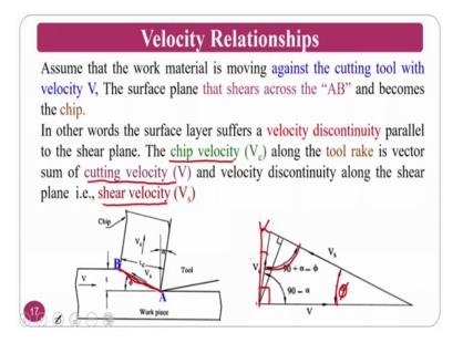
Assume that the work material is moving against the cutting tool with the velocity V that is the cutting velocity. The surface plane that shears is AB; that is what I am saying this is the plane shearing plane which is nothing, but the V s.
