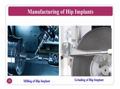
Hip implant also can be manufactured by the machining process, the whatever you have seen in the previous one is a forming process here. You can also do this particular, hip implant by the machining process. You can see here, the profile milling is taking care by the machining operation, followed by. You can also do the grinding operation; you can see the grinding wheel, which is very thin. Grinding wheels are used to generate the some profiles on the hip implants.
