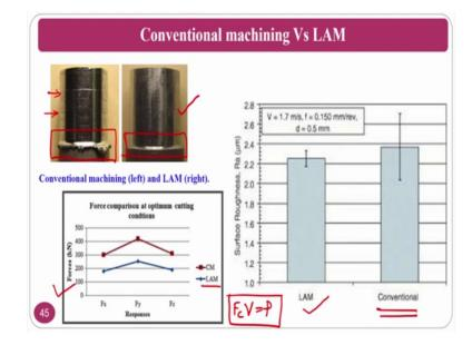
You can see here the forces or the surfaces. Normally, here you can see how the burs are formed; no burs are formed at the same time. Good surface finish is achieved, compared to this one; you have a line here, line here and all those things; that means, that surface quality in laser assisting machining is much better, whenever you are doing the machining operation for the brittle materials or very hard materials and all those things.
