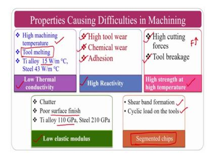
So, properties causing the difficulty in machining the first property; is as I said lower thermal conductivity; If the thermal conductivity of this particular material is 15 and high machining temperature during the machining process. If the temperature is very high, it cannot conduct the temperature inside the workpiece material. So, it will impart to the tool. So, the thermal softening of the tool takes place and tool melting will takes place thermal and tool will fail.
