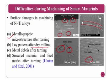
So, metallographic microstructure, after the one you can see here, wherever the surface cavities are formed and all those things and the carbide particles also stays here ok. Whenever people are using here, nickel titanium alloys are more one of the common examples for the smart materials.
