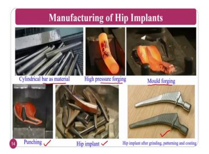
If you want to do the hip implant basically, if you see the hip implants first, cylindrical bars as a materials, you can take, then high pressure forging will be done for the giving shape, then mould forging will be done. That is the, whatever the shape of the mould, that you can generate, then will be the forging operation, then you can do the punching to an extract that component.
