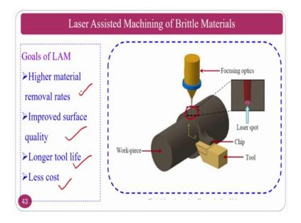
The schematic view, if you see here, the laser is falling here, this is our own picture, we have drawn especially for you. So, laser is falling here and ahead of the turning position. This particular portion is softened and, and then you are removing the material in that circumstances, the cutting tool experiences low forces. So, it can easily remove the material, that is high material removal rates improve, the surface quality tool life will improve and the less cost ok.
