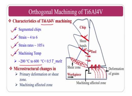
So, the characteristics of Ti 6 Al 4 V, this is the one of the common material that aerospace industry uses. So, segmented chips, you are going to get strains, are approximately 4 to 6 strain rates are 1 naught 5 for second, the machining temperature will be very high, that is 200 to 600 degrees and you can see here, the primary deformation zone and the machining effected zone.
