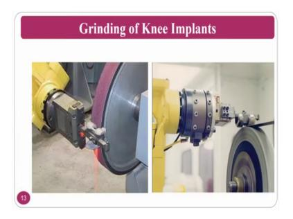
So, at the same time, if you want to fabricate, the component are the knee implant at the minimum price. You can go for the belt grinding or buffing operations also ok. So, advanced finishing processes like what I said MRF or magnetorheological finishing or ball end magnetorheological finishing, this type of processes assume that these are going to be costly for you, then you can design your own belt grinding process and all those things like, what is given here.
