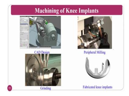
If the first procedure will be goes like this. First, you have to design, a CAD design model then, you go for the machining operation, you can see here, the peripheral building is done at the same time. You can clearly see here, it is ball; end type of milling is done. So, that the surface finish will be better, then you can go for the grinding operation and you can see the final product, how it can be fabricated?
