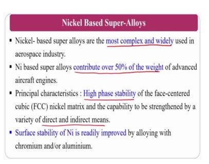
Nickel based super alloys, nickel based super alloys are the most complex and widely
