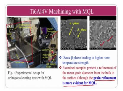
This is the machining setup. To avoid up to certain extent, people have used here minimum quantity lubrication or the minimum quantity cuttings fluid, if this is the machining zone, where the machining zone is taking place and you can see the infrared camera is focused. Lubricant pressurized is also given and all those things and dense beta phase, alpha phase, all you can see here, but the thing what the people experience are reported in this.
