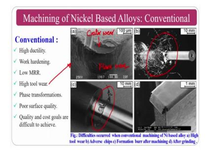
The machining of the nickel based alloys conventionally. So, high ductility work hardening low material, removal rate high tool wear. Basically, it is a super alloy material in that circumstances, the tool wear will be very high, the phase transformations will takes place quality that you are going to get on the surface is very poor and the cost goals are difficult to achieve quality and all those things ok.
