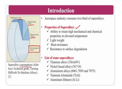
Mostly, super alloys are used in the aerospace applications, if you see super alloys consumption in the market, the structural application is 10 percent, chemical industry 10 percent, medical industry 10 percent, but aerospace industry is 70 percent. That is why super alloys like, nickel based alloys and all those things are play a major role in the aerospace industry. That is why we see how to machining the super alloys? What are the problems and we also see the other materials also.
