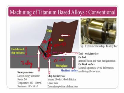
If we see the machining process, it is looks like a ductile and material, because it is a soft material. Even though it is a super alloy type of material, but it, it is a basically a ductile material. That is why, you always see a thick zone ok. You people have studied already thin zone models and thick zone models. If the shear plane is like a line, it is thin zone model.
