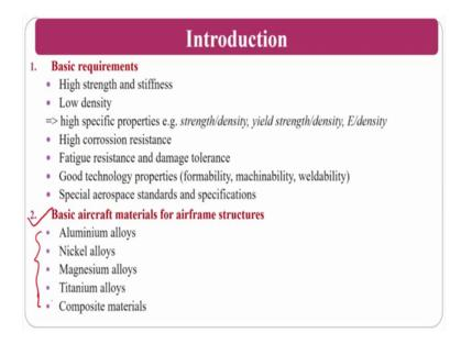
Now, we move on to the machining of aerospace materials. So, aerospace materials; the basic requirements goes like many things and the basic aircraft materials here from structures and all those things. Normally, these are the materials that are used in this one, a properties of the superalloys.
