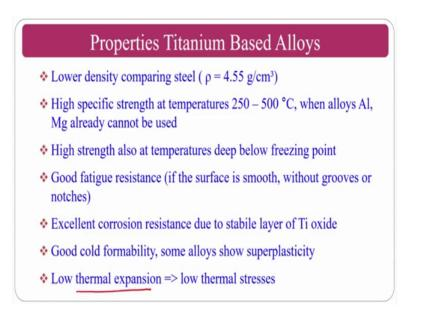
The properties it will have a lower density, comparing to steel high specific strength at elevated temperatures, also high strength at temperatures below the freezing temperature
