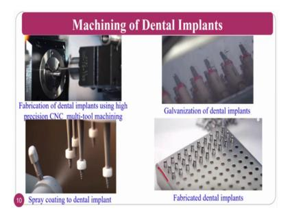
So, machining of dental implant; the procedure goes like this. First, you just fix the dental implant material. Normally, this will be done on the titanium, then using a CNC multi-tool machining process; just you do the turning operation. Normally, patterning operation and all those things, then you generate the threads as per your requirement, then you can do the post processing like coating and all those things also.
