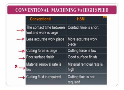
Conventional machining versus high-speed machining, what are the differences? in the contact time between the tool and workpiece will be large in convention, because you are speed is low. If the speed is low for the particular length of a workpiece material what will happen, the contact time will be large, and in high-speed machining contact time will be less; So, less accuracy of the workpiece.
