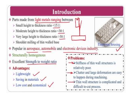
Wall machining has a great applications in various sectors, especially electronics sector. If you open your CPU, basically you will find 2 or 3 thin walled components for taking out the heat dissipation in the CPU. The parts made up of light materials ranging between small height to thickness ratio that is called 15 is to 1, moderate height with thickness ratio 30 is to 1, very large height to thickness ratio 30 is to 1 above 30 is to 1. So, shoulder milling and all those things.
