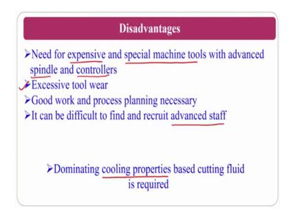
See there are some disadvantages of high-speed machining also. So, you need an expensive and the special type of machine tools, because whenever you operate very high speeds the chances of that machine is that it can vibrate. So, you need a precise machine tool, for that purpose you need to have the advanced spindles and controller. At the same time if you take care about your machine tool dynamics and all those things.
