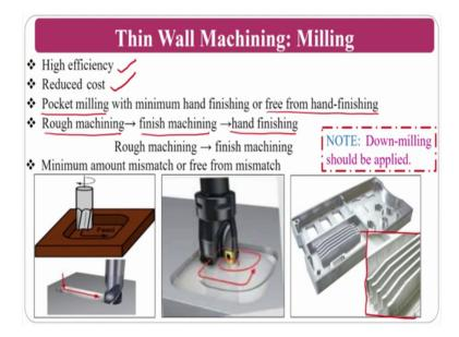
So, thin wall machining, basically you can do by the milling process, whenever you do the milling process high efficiency reduction cost, pocket milling with the minimum hand finishing or the free form hand finishing you can do, and the rough machining also followed by the fine finish machining, then the hand finishing and these are all the some of the techniques that people are going to use for making the thin walls.
