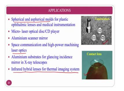
The applications, if you see the applications normally the contact lenses, moulds, the camera lenses moulds, these are the things can be manufactured by this particular process; spherical and aspherical molds of this particular ophthalmic lens and medical instruments can be prepared micro-laser optical disc, CD players will be and aluminium scanner mirrors.
