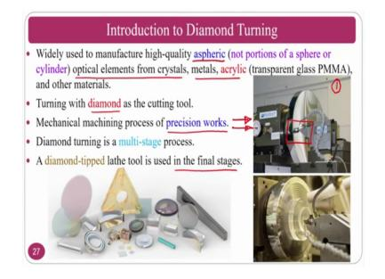
Now, we move on to the diamond turning. So, how the diamond tools are fabricated and all those things we do not see, but if you see particularly, the mirrors. If you see the figure 1 the mirrors are finished by using the diamond turning operation and these are the components, super quality finish. Normally, these diamond turning is costly process, because you are tool itself in this particular process is a diamond one.
