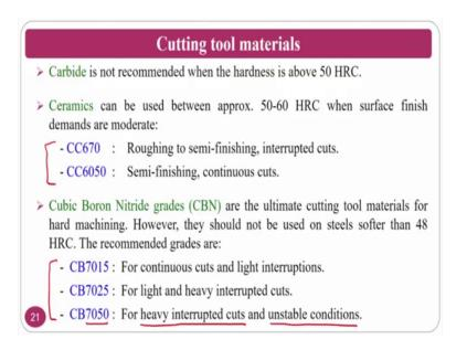
The cutting tool materials carbide is not recommended when the hardness is above 50 HRC. At the same time ceramic tools are preferred. These are the codes of some companies where the people will use for the continuous, discontinuous and all those things. Cubic boron nitride is a mostly preferred one, as I said from the previous one.
