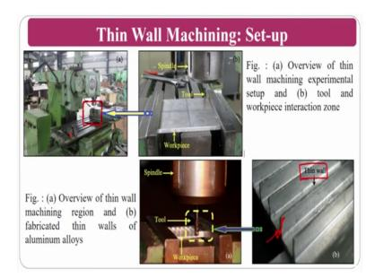
If you see this is a particularly we have tried to take the pictures using aluminium, copper which are the soft materials and you can even see here that the thin walls that are machined here in this particular thing is the aluminium alloy, where the thickness is approximately 1 mm, but I cannot say this is the thin wall machining process, but still we
