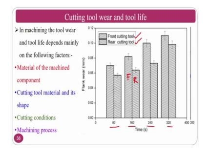
The cutting tool wear life and all those things. Normally the tool wear if you talk in terms of the front and the rear tool. Rear tool; obviously, the flank wear will be very less, because the workpiece is getting thermal softened and all those things. In the machining the, if you talk about the tool wear in the front cutting tool and the rear cutting tool, the tool wears normally if you talk. The front tool wear will be slightly higher, because you are removing the original material.
