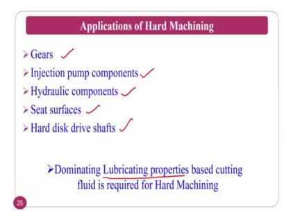
So, applications of the hard machining, normally these are all used for the gears application, injection pump application, hydraulic components, seat surfaces, hard disk
