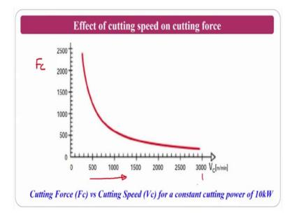
If you see particularly about the cutting force versus cutting speed, e as the speed is increasing what is happening? The cutting force basically Fc is gradually decreasing, but this is up to certain velocity. Whatever you have seen the previous graph is beyond the range that inner zone.
