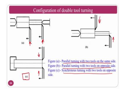
So there are three varieties; one is a parallel turning with two cutting tools on the same side, one is here, another one is here. This is the one. The second is parallel turning with two tools on the opposite direction; one is here another one is here.
