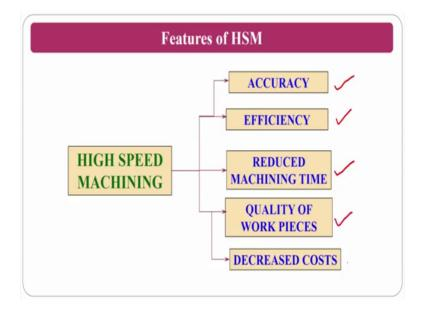
If you see the features of high-speed machining, the high-speed machining, the features you will get is good accuracy and the efficiency, because you are going to machine many parts in less time, because your speed is very high; that means, that you are efficiency or the performance is very high, reduced machining time, because you are machining at very high speed, so the part to be manufactured will take very less time.
