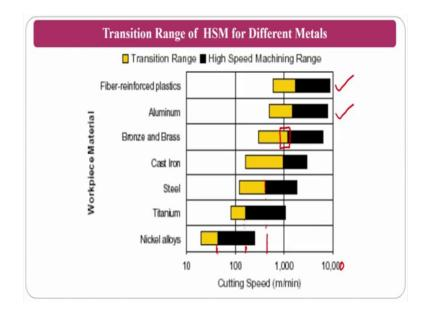
So, various materials will have various transition ranges of high speed machining, because if you take a aluminium, if you take the hard steel, both assume that if I am rotating for that same RPM tool with help of head stock. You cannot say the same is considered as a hard machining. In steels, hard steels you may consider as hard, high speed machining, but not in case of the aluminium, because there is a hardness variation ok
