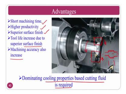
Advantages of this particular process; short machining time, because you are doing with two tools high productivity and superior surface finish subjected to the machining conditions. Tool life increases due to superior surface finish. Tool life normally will be increased in terms of the rear tool, machining accuracy also increases. This is about the advantages.
