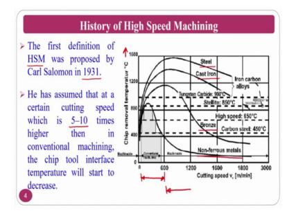
If you see the history the, this is the first definition of high speed machining was proposed by Carl Salomon in 1931. Later on what happen it has the assumed that the certain cutting speed which is 5 to 10 times higher than the conventional machining processes, where the chip tool temperature goes down; that is what the proposed thing and that it was the some of the people they have invented.
