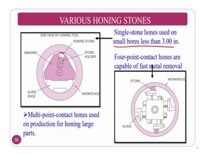
Various honing stones it is called a single stone with the small bore normally you will have only single stone that is going to finish because it will goes rotates and goes inside reciprocate. So, you can do and the multiple also. So, in whatever you have seen in the previous slide where there are 4 that is called multiple type. So, you can if at all I want to remove more amount of material you have to go for multiple storms.
