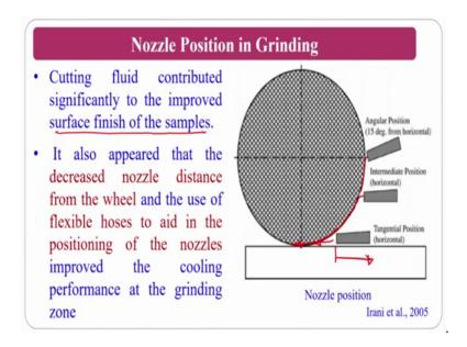
Nozzle positions in the grinding if you see there are some researchers working on or worked already on the nozzle positions, you can use tangential position at the same time you can use intermediate position because you need certain boundary basically what will happen if you are using here the cutting fluid goes like this. So, it will occupy the machining region if you use here what will happen it comes through the boundary and goes like this ok.
