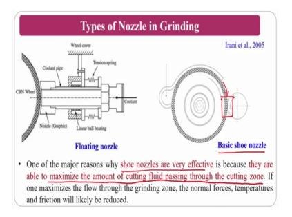
So, the types of nozzles if you see the first one is the basic shoe nozzle this is the one of the common and commercial type of thing, where if you see normally this shoe nozzles are very effective because they are they able to maximise the amount of cutting fluid passing through the cutting zone this is the cutting zone. So, this a workpiece interface and the grinding wheel interface. So, that it can pass through the grinding fluid and it maximise on the periphery of the machining region.
