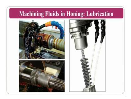
The lubrication are the cutting fluids in honing process mostly the cutting fluids here we will be used is lubricants, as you can see here these are all mostly lubricant type of cutting fluids will be used. So, water base cutting fluids are not used if at all used very less amount of water base, because a cooling is not a criteria here the lubrication is the major thing that the people want here.
