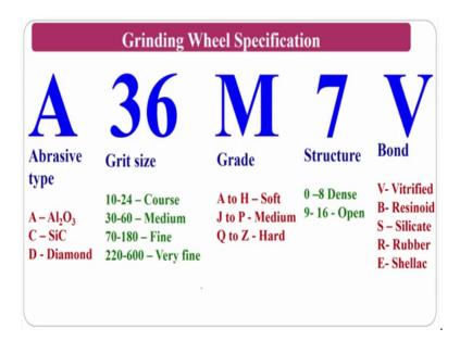
But as you have already seen the grinding wheel specification in this one, which is the most important one that will have influence with respect to the grinding fluids that we have to see as abrasive type you do not have any much thing because whether it is alumina or a silicon carbide or diamond whatever the things. So, whether is a grid size you know it will have much effect because what are the grid size you are using whether it is you are using medium or coarse or something.
