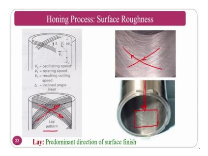
Surface roughness if you see as I said the crosshatch pattern will be generated on the engine cylinders or the cylinder liners, whatever you are seeing here this is the lay that is nothing, but predominance direction of the surface roughness or the surface finish you can see the this is reverse direction and this is going direction.
