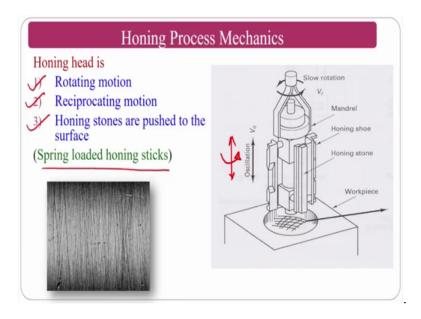
The honing head it will have a rotating motion it will have a reciprocating motion honing stones are pushed to the surfaces by the spring loading honing sticks ok. So, that you can
