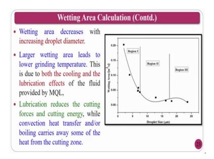
The same thing is reflecting here the droplet size versus wetting area as the wetting area as the wetting area as the droplet sizing increases what will happen the wetting area is decreasing. So, wetting area decreases with increasing droplet the larger wetting area leads to lower grinding temperature ok. If you can if you can decrease this one particle size or the droplet size you can occupy more area and more area. So, that temperature of that particular area you can take out easily.
