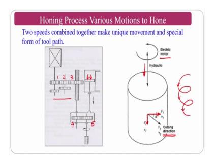
How you can give or the impart the rotary motion and as well as the reciprocation motion, rotary motion is transferred with respect to gears this gear 1 to gear 2 to gear 3. So, that you can transfer this to the gear 4 and you can transfer to the gear 5, but the same time reciprocation motion you are going to get from this ok. So, indirectly you are going to get the rotary motion as well as reciprocation motion, then if you can synchronise both you will get a helical path.
