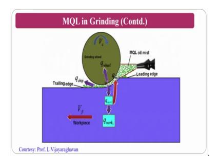
This is how you can see here the grinding wheel and the minimum quantity lubrication the fluid is occupying here and the abrasive particles will be there and this will remove the workpiece material ok. These slides are taken from one of the senior professors from IIT Madras so, thankful to the professor.
