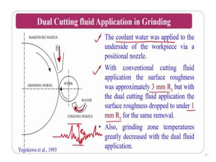
There is another nozzle type that is called dual nozzle which we have seen the schematic in the previous slides. So, here also you can use the coolant there is oil which is coming from here at the same time there is a water also coming from here dual nozzles are there the oil will help in lubrication at the same time water will help in cooling.
