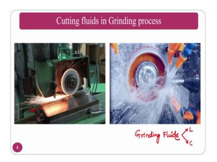
The grinding fluids basically if you see in a machining operation other surface grinding, here in this region you can see lot of spark is generated because of the friction that is between the grinding wheels as well as the workpiece surface. So, in order to reduce the temperate generation and the heat affected on the workpiece and all those things always people will use the grinding fluids.
