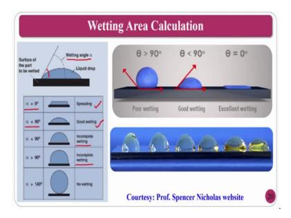
Wetting area calculation this is the another important area, where whenever the droplet us are falling in the machining region whether it is occupying the complete area or it is not occupying the complete area that is one of the concern for that purpose you have to play with your particular cutting fluid.
