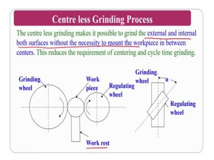
Centre less grinding is another variety of grinding process, where there are two varieties one is given here, this is a external and internal both surfaces you can do by this centre less grinding process; that means, that there is no center if at all I want to do the
