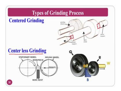
So, two things are there one is centered grinding as well as centre less grinding, if you see here in the centered grinding there it is the work piece held between the centers. So, perfectly only I can do it for the normal regular shape, if at all I have a irregular surface, then I have to go for center less grinding process that I have told in the previous slide also.
