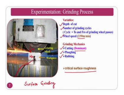
If you see this particular process, where the shown is surface grinding, what is surface grinding and other things you will come across so, the surface grinding just there is a work piece, this is the work piece and, this is a wheel the wheel is rotating at certain speed 2350 per RPM, it is rotating it is taken from the laboratory or laboratory only. So, various variables that you can give and you can generate, or you can get the output responses.
