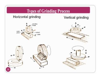
So, types of grinding if you see horizontal grinding vertical grinding in as you see, in the milling process also you will have the horizontal grinding and vertical grinding where the your Arber axis where you will mount, if it is parallel to your work piece that is called horizontal, if it is perpendicular then it is called vertical.
