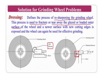
Now, how to resolve this problems these are the common problems of the grinding wheel and, the solutions if you see here one is dressing. So, dressing defines the process of re sharpening of the grinding wheel this process used to fracture or tear away, the glazed or loaded outer surface that means, that it is applicable for both the problems that is the glazing, if you see the glazing that mean that the sharp edges are gone and it becomes smooth on the wheel.
