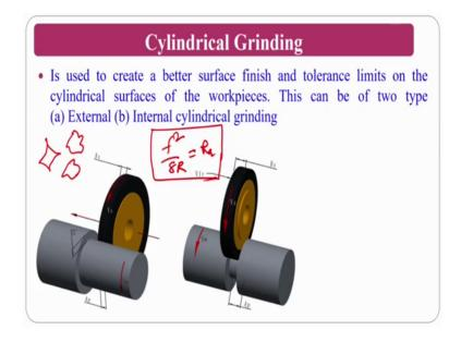
Cylindrical grinding is another one where you can see here, if at all I want the good geometry you can get even by turning the operation also, but the problem with the turning process is your surface roughness that is f square by 8 R equal to your R a will be; that means, that it is will be a function of your feed as well as nose areas here, there is nothing because your abrasive particle is too tiny and it will remove the material.
