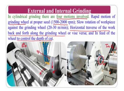
So, external and internal just if you see that is a schematic diagram, these are the practical diagram, that is the schematic diagrams and this is the practically visible diagrams that we have taken. So, if you see cylindrical grinding process there are 4 motions which are involved in the cylindrical grinding process.
