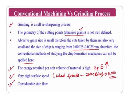
Thus it that is about the grinding. So, the conventional machining versus grinding process if you see the grinding is a self sharpening process, self sharpening process means if the abrasive are gone. So, new abrasives will come into picture that is nothing, but the grinding wheel is a brittle material basically, if a set of particles are assume that I have a grinding wheel like this.
