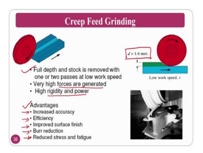
There is another variety which is called creep feed grinding where the depth of cut is so, high. Normally so, if the full depth of cutter stock is removed in one or two process, normally it is called as a creep feed grinding and very high forces are generated and very high rigidity and power is required in the grinding wheel for this one.
