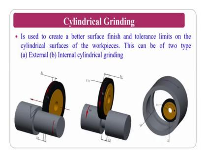
If you see there is another cylindrical process that is called internal cylindrical process, if you are working on outside surface it is external cylindrical grinding process, if you are working inside that is called inner cylindrical grinding process.
