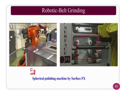
If you see there is second variety there is also grinding wheels, which where you can put the complex surfaces using the robotic arm, here also not only the belts you can also use the grinding wheels itself that is what I want to show, if you see here the second picture this is the figure 1, where hip implant stem is fabricating, or finishing is going on.
