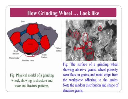
These are the grinding abrasive particles these are the abrasive particles and, this is the bonding and in between there is a porosity and all those things this is a schematic diagram, this is the physical model or how you can represent that one under you can also see attritious wear and all those things here. So, if you see practically how it look like these are the voids, this is the bonding this is the abrasive particle this is the abrasive particle in between you have a bonding.
