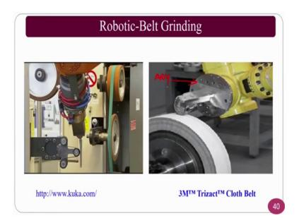
So, here you are use the robotic arm to against the built grinding process, if you see here it is a hip implant basically machined against the built grinding process ok. These are the belt, if you see this is also belt and this is also a belt continuously flowing belt is there which is moving and.
