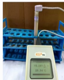
Thermal conductivity and specific heat measurement setup
