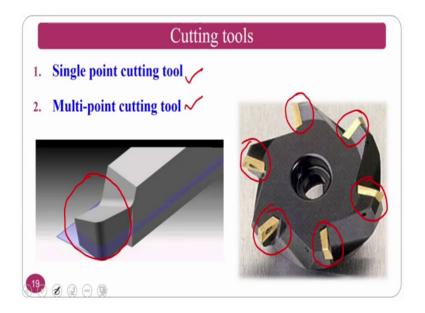
So, in the cutting tools basically we study about 2 varieties of cutting tools. One is single point cutting tool, and multipoint cutting tool. This is simply you can see. This is a single point cutting tool. Normally lathe machine turning operation and all those things operates on single point cutting tool.
