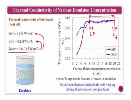
Thermal conductivity of the lubricants normally mineral oil if you see mineral oil thermal conductivity of the mineral oil is 0.126, but the bio cutting fluid is 0.151.
