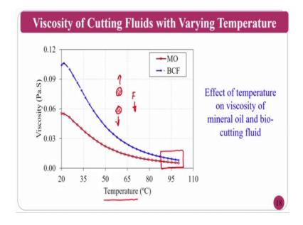
Now, we will see about the variation in with respect to temperature, if you see the variation with respect to temperature both the fluids are decreasing with respect to temperature; that means, that whenever you are increasing the temperature the particles in two particles intermolecular distance is going to increase with respect to temperature; that means, that intermolecular force of attraction goes decreases that is the viscosity gradually decreases.
