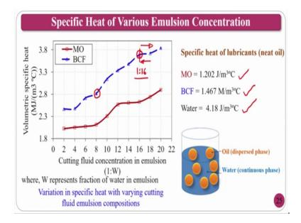
Now, we will see the specific heat one the specific heat of the lubricants mineral oil is 1.2 bio cutting fluid is again 1.467; that means, approximately 1.5, but water will have higher that is called 4.1 or 4.2 approximately.
