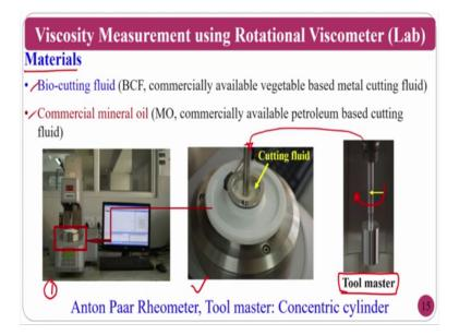
So, this is how the experiment will takes place, but this is for the semi solids and all those things normally you will use the parallel plate rheometer, but if at all somebody want to do the radiology of the liquid normally plan parallel plate is not used. Whatever we have shown in this particular slide is to explain you how the physics of the rheometer goes on? That is what we want to say for that purpose easily understanding is by the parallel plate rheometer ok.
