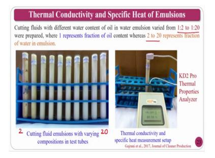
So, now we have to check which is having the good thermal properties for that purpose what we have done here is the emulsions are mixed from 2 to 20 a percent of the that is one is to 2 to 1 is to 20. So, 1 litre of cutting fluid to the 2 litres of water ranging from that to 1 is 1 litre of cutting fluid to 20 litres of cutting fluid.
