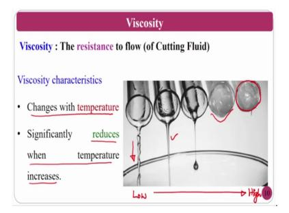
The viscosity is nothing, but the resistance to flow of the cutting fluid, if you see here in this particular picture the viscosity is low here and the viscosity is high here. For the same inclination or something whatever is given the flow rate that is falling from the test tube is gradually increasing from this to this that is why the viscosity is gradually increasing.
