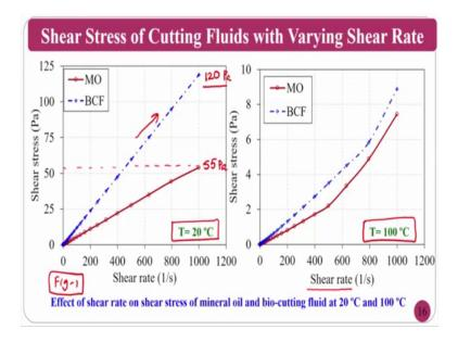
Shear stress if you see the shear stress versus shear rate in for the mineral oil as well as bio cutting fluid, the shear stress required for the bio cutting fluid is higher compared to the shear stress required for the mineral oil based cutting fluids. Normally it required around 55 and this requires about 120 or something 120 Pascal and this is 55 around 55 Pascal at a 20 degrees. What it shows it shows that bio cutting fluid is much viscous compared to your mineral oil ok.
