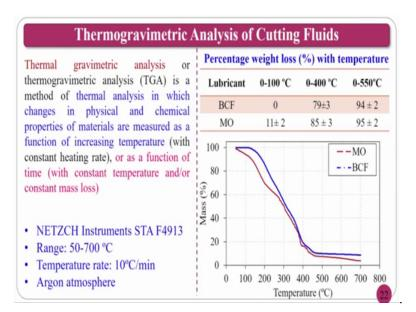
Here we will see the thermal conductivity and specific heat about the emulsions and all those things, thermal gravimetric analysis of the cutting fluid, if you see TGA is a method of thermal analysis, which changes the physical and chemical properties of materials, measured the function of increasing with respect to temperature.
