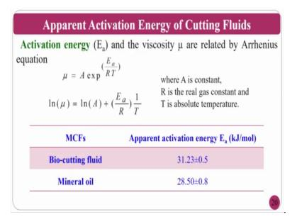
If you see the apparent activation energy of the cutting fluid the relation between the activation energy and the viscosity are related by the Arrhenius equation that is called mu equal to a into exponential of E a by R T, where A is a constant R is the real gas constant
