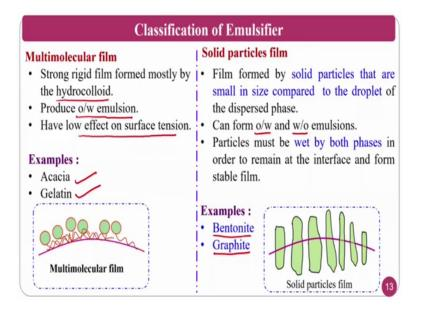
Multimolecular films emulsifier strong and rigid formed a mostly by the hydrocolloid as I said colloid. Emulsifier is liquid to liquid here if it is semi solid to liquid or solid to liquid normally it is called less colloid hydrocolloids. Normally if you might people might have heard about hydrogels, gelatin hydrogels, t e g hydrogels, p l e hydrogels , or p e g p l e p g hydrogels, there are hydrogels, hydro gel.
