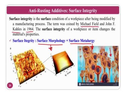
So, surface integrity, I was just talking about the surface integrity and surface roughness I have already taught you. But I forgot to give you some other glimpse that is called surface integrity is surface condition of the work piecebeing modified by the manufacturing process the term is coined by the Michael Field and John F Kahles in 1964. Surface integrity means surface morphology plus surface metalurgy ok. This is about the surface integrity.
