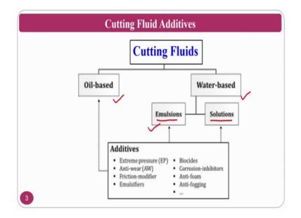
If you see the cutting fluids there are two types of cutting fluids normally metalworking fluids are the broadly says this word, but cutting fluids are specified words. So, cutting fluids are one part of metalworking fluids. Metalworking fluids even metal forming across some of the grease is they will use, some of the lubricants they will use those are
