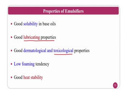
Properties of emulsifiers, normally it should have good solubility in base oil. Base oil means if you can mix with base oil then you can mix with water or you can normally the cutting fluids a lubricant whenever you purchase from the market it will be already blended inside the mineral oil. So that means, that it should be completely lipophilic lipophilic as I said that this completely emulsions are lipophilic it should uniformly mix
