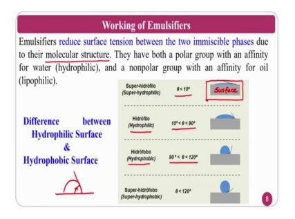
So, I was talking about hydrophobic and hydrophilic surfaces and all those things. Emulsifier reduce the surface tension between two immiscible faces due to their molecular structure ok. Because of their molecular structure that is called polar and nonpolar they have both group and affinity towards water that is called nonpolar group is affinity water and forms the molecule.
