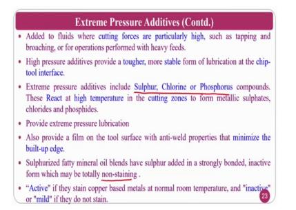
Added fluids where the cutting fluid forces are particularly high such as tapping and broaching operation (Refer Time: 43:12). These are applied for heavy load processes where the cutting forces are high like broaching operation you need to have lot of forces during the machining operation.
