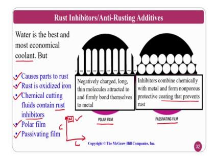
So, water is the best and most economical coolant ok, because it is freely available at the same time cost free and it has if you see the graph it has a better cooling ability. If you see the graph like lubrication versus cooling abilities water stays here ok. So, for that purpose this is a better coolant and it has no charge ok.
