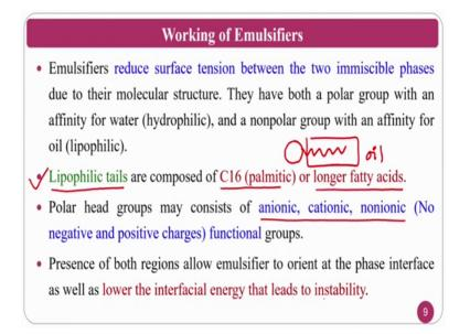
So, we now move to the emulsifier reduces surface tension between two immiscible phase due to their molecular structure. Lipophilic tails are composed of normally C16 that is longer fatty acids. What is lipophilic tails? Lipophilic tails means, lipophilic
