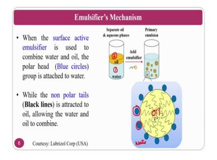
This is about the mechanism. However, we will go into the complete mechanism when a surface active emulsifier is used to combine with water and oil if you see in the picture. So, normally this blue circles. This blue circles are nothing, but you are polar molecules is attached to the water; that means, this blue one is water this is oil.
