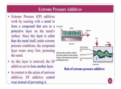
So, extreme pressure additives a work reacting with a metal form a compound that reacts a protective layer on the metal surface. Since this layer is softer than metal under extreme pressure conditions it bears of protecting in the metals. That means, whenever extreme pressure additive is added to the cutting fluid if it is falls during the machining operation what will happen it forms a layer that is soft compared to my parent material of that material.
