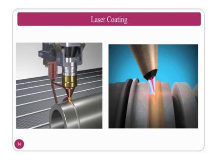
Not only on tools you can also do on various materials because nowadays it is becoming one of the important process because laser has very flexibility the huge flexibility of the laser will help in proper coating and proper bonding in the material ok.
