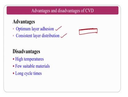
So, the advantages if you see the optimum layer adhesion will takes place and consistent layer distribution will takes place. Suppose that uniform layer will takes place on a substrate if I have a substrate uniform layer will takes place on this one without any disturbance ok.
