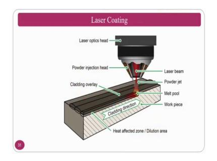
So, that is one of the beauty and you can see this is the cladding direction or what are the other things like a laser beam is there, powder jet is there this is the coaxial powder system is there melt pool is taking place and a workpiece ok.
