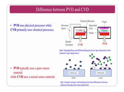
So, if you see the difference between PVD and CVD; till now we have seen many {VD varieties only we have seen the CVD only one. So, PVD uses physical source while CVD primarily uses a chemical process; so, that is a different.
