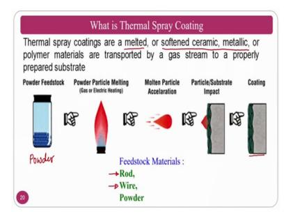
So, what is the thermal spray coating ok? So, the thermal spray coating thermal spray coatings are molt melted softened ceramic or a metallic polymer materials are transported by a gas stream and the property that is what I was telling.
