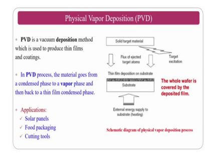
Now, we are coming to the physical vapor deposition ok. Physical vapor deposition done normally in a vacuum ok; it is done in the vacuum method which was used to produce the thin films or the coatings on the substrate material ok. So, in here schematic is here the in the PVD process the material goes from condensed phase to the vapor phase again come back to the condensed phase in the form of thin material ok.
