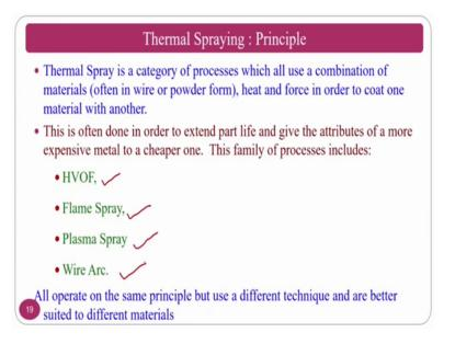
If you see thermal spraying is one of the most thick coatings if at all you want thermal spraying is one of the techniques ok. Thermal spraying categorized as a one of the combination material heat force in order to cope ok.
