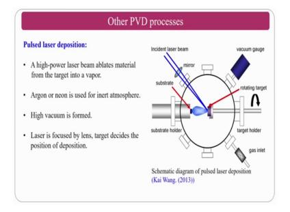
Other PVDs are pulsed laser deposition where high power laser beam ablates a material from the target whenever they you just send the high less power beam on the target what will happen? It will ablate the material is that it will become the vapors. Argon neon gas is used as a inert atmosphere and a high vacuum is formed and laser focused on lens and decide the position ok; now it will decide the position and it will deposit on top of it.
