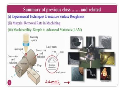
So, the other thing we have seen in the last where we end yesterday was a laser assisted machining; schematic diagram would have been a better option, but I have shown you some of the applications of a laser assisted machining those who. So, to brush up you how the laser assisted machining will be there. So, this will be a laser source which imparts a laser beam on this one and you can heat it.
