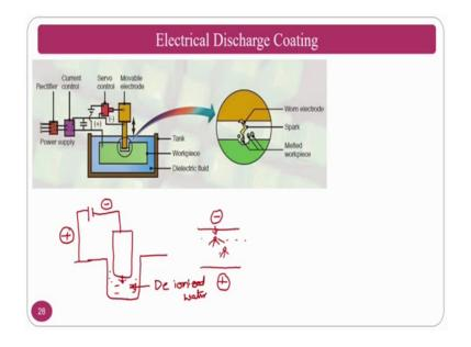
So, normally electric discharge machining many of you may know from the point of electric discharge machining ok. When the electric discharge machining will takes place electric discharge machining, normally you will connect the negative terminal to the tool and the positive terminal to the workpiece ok. So, the electrons start flowing from assume that I have a same schematically draw here if this is the just a schematic where my tool is there ok.
