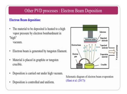
So, electron beam deposition also you can take a metal deposited it is heated to a high vapor pressure by electron bombardment and in the vacuum the electron beam generated by the tungsten filament normally tungsten filament is used to bombard and then the deposition is carried out in a vacuum and the beauty about this is the uniform coating will takes place ok.
