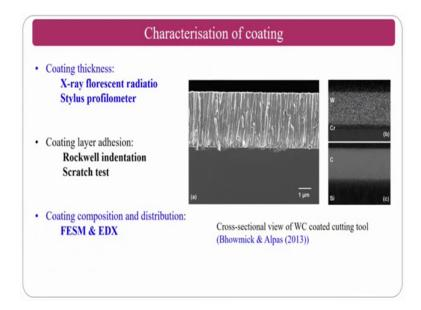
So, characterization of coatings is another big area which we have already seen. So, X-ray florescent radio stylus profilometer can be normally used; at the same time you can use 3D profilometers also to measure the thickness of the coat and all those things.
