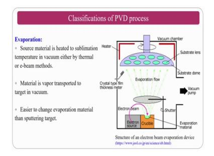
So, classification this is the evaporation techniques where the source material is heated to the sublimation temperature; then the thermal by the e beam method and then you can coat on the substrate material where you want to coat ok.
