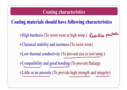
The coating materials should have following characteristics; what are the characteristics that I want whenever I am coating for particular machining application high hardness I said know very resistance hardness.
