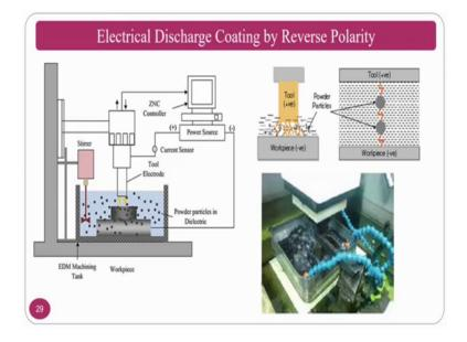
So, if you mix along with that one the powder mix that is what I was telling; if you do the powder mixing is done whatever the material that I want to coat in a dielectric fluid plus if I do the reverse polarity where ions and electrons interact change between workpiece and tool what will happen? There is a deposition takes place and the deposition these particles also play a major role. So, that the deposition may be better
