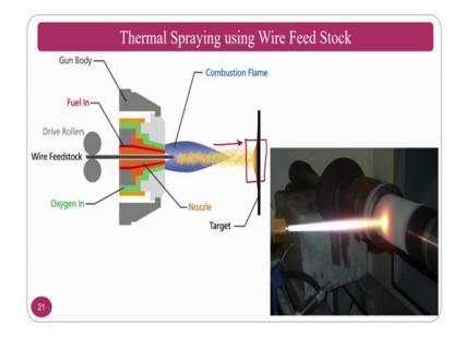
If you see the wire feed previously we have seen a powder now we have seen the wire feed stock if you are using the rollers drive rollers and just you feed it; now the fuel is in and if it is melting then you are sending with high pressure. So, you will get a coat on the target material this is the my target; where this molten material is going and adhering to the surface ok.
