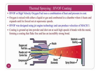
Then comes another thermal spraying techniques that is called HVOF coating that is called the high velocity oxy fuel coating ok, where here you will use the heat and pressure to cope ok. So, you will also use the heat that to melt the material that you have to coat on top of it and uses the pressure to coat on it. Oxygen is mixed with a liquid or a gas and combustion chamber will heat until the force at the supersonic speeds like mach 3 ok.
