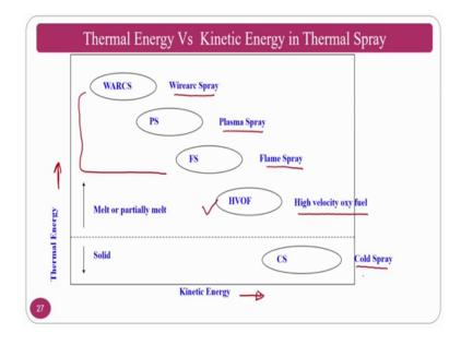
If you see the kinetic energy versus thermal energy; normally the thermal energy requirements are very high for arcs spray followed by the plasma spray, flames spray and high velocity oxy fuel and all those things ok.
