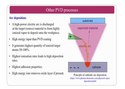
So, other PVD techniques is arc deposition technique and the high electric arc discharge at a target from the highly ionized vapor will come and deposit on the material ok.
