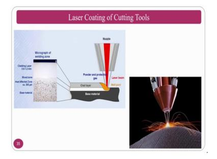
So, this is a another way of the coating you can see the laser coating area. So, the base material is there if you do the cross sectional study of this one the mixed zone is there, heat affected zone is there and cladding zone is there this how you do the cladding and
