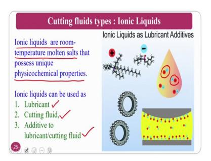
Ionic liquids as a lubricant addictive I already said these are the liquids ionic liquids at room temperature and molten salts ok. So, this process from physio chemical properties
