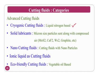
So, we now proceed to the solid lubricants and the nano cutting to fluid ionic cutting fluid ecofriendly cutting fluid.
