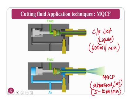
So, in the normal condition is high pressure cutting fluid jet this one if you use MQCF jet ok. So, you can see here normally the it will be a liquid here, here it will be a atomized jet, ok, well good, ok.
