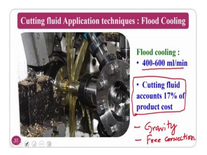
So, the first one is flood cooling where you can see the coolant or the lubricant that is flowing like a water that if you pour water from a glass it is ok. So, by virtue of gravity it falls ok. So, it falls in the machining region by the virtue of gravity ok.
