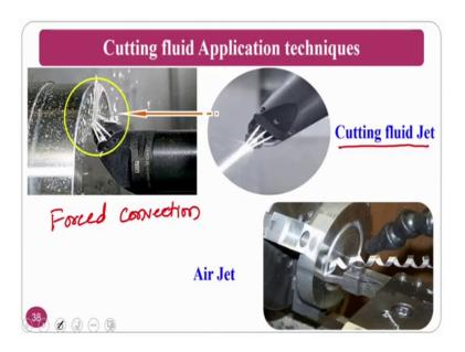
So, second one is jet application cutting fluid jet application ok. So, where you can see here where the high pressure jet is send or into the chip tool interface. If you see here chip tool interface it is sending in the machining region. Normally here in the flood cooling it is by virtue of the gravity it is falling here you are pumping with very high pressures, so the convection will be higher side to the flood cooling. But the advantage here is forced convection ok.
