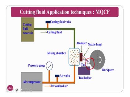
You can also do the internal mixing of these things. So, if you see the cutting fluid reservoir will be there and you are sending the cutting fluid and you are sending air compressor air just you mix in the mixing chamber then you just divert into the machining region ok. This is the internal mixing.
