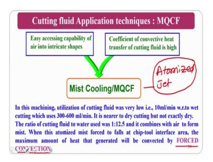
Let me explain you in one case what I am getting is easy accessible capabilities of air into intricate shapes; that means, I am using a highly compressed air which has can enter into the intricate regions of my metal cutting I mean to say if this is the metal cutting. So, it can enter like a jet it can enter like a jet.
