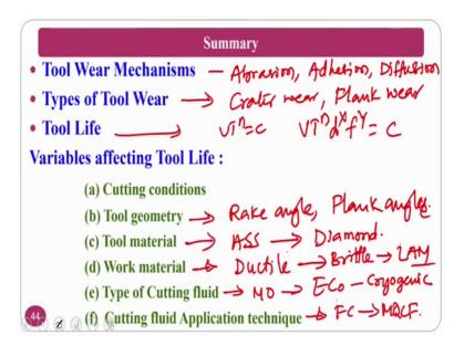
So, let me summarize. So, we have seen in this chapter tool wear mechanisms, tool, types of tool wear that is crater wear and flank wear, tool wear mechanisms such as abrasion, adhesion, and diffusion. Tool wears, normally two tool wears one crater wear, two flank wear.
