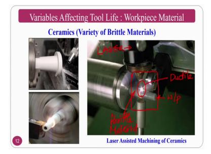
So, I have a work piece material, this is the work piece the tool is cutting from the other side, this is the laser source this is a laser. So, if the beam is falling here you can see in this machining region.
