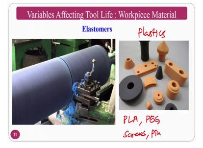
So, whenever you do the machining, if it is elastomers and all those things it has it is own drawbacks, because if I give a certain depth of cut. Because of the elasticity of the work piece material it may deform, some material may come in the particular depth of cut, some material may not come if I am giving 5 microns, the cut maybe 4.5 or something, there will be a some deformation will takes place and all those things.
