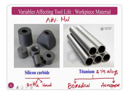
Anyhow this is just a overview t, we just go into the different materials that we come across. Silicon carbide is one of the ceramic material, it is very difficult to machine the ceramics, because these are the brittle materials and hard materials.
