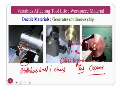
Now, coming to the ductile materials, the first variety of the work piece materials are ductile materials. Normally the leopard material ranging from stainless steel, this is a stainless steel and this is the copper. So, the stainless steel are with iron based steals. So, machining this normally generates the continuous chip, as you can see here it generates the continuous chips.
