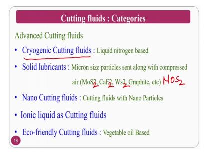
So, MoS 2 CaF 2 that is Calcium Fluoride and Tungsten Disulphide. So, these are the common lubricating properties, even graphite also. Just you make a power of this, which are the lubricating properties and you send along with a highly compressed day.
