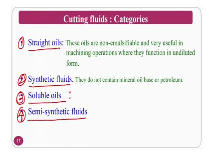
So, there are varieties of cutting of cutting fluids. 4 basic styles are there one is strait oils and the synthetic fluids, soluble oils and semi synthetic fluids these are the 4 varieties.
