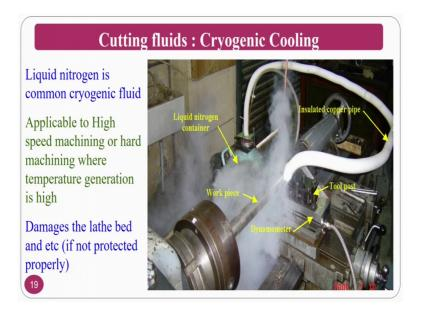
So, normally used is liquid nitrogen in the current photograph whatever you can see is the liquid nitrogen based cryogenic machining, where the cryogenic fluid is as a coolant basically. It is a better coolant, because the temperature is minus 164 degrees, normally minus 160 degrees is a temperature.
