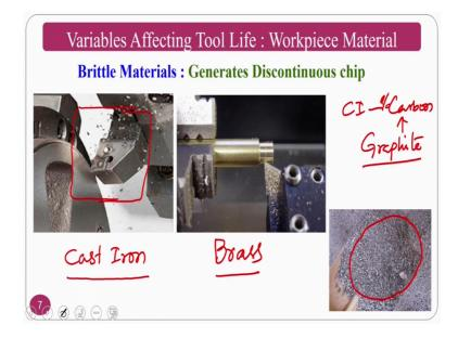
So, carbon in the form of graphite graphite if you see nowadays people talks about graphing and all those things. So, the graphite act as a self-lubricant basically. So, whenever you drill a hole in a cast iron, whenever you do machining like if you see for example, here cast iron is machined here.
