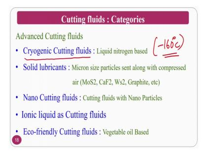
Whenever we want to go for the advanced versions, these are the advanced version of the cutting fluids. If you see the first and foremost is the cryogenic cutting fluid, normally cryogenic cutting fluid is nothing, but a liquid nitrogen based fluid. This is basically used for high temperature applications, wherever if at all the Titanium is machined are ceramic materials machined and all those things.
