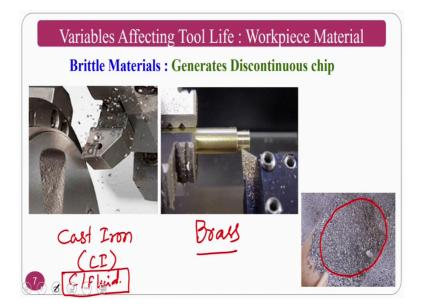
So, whenever we are going to the brittle materials, ductile materials will give the continuous chip, but the brittle materials normally the basic examples of the brittle materials is the cast iron. The first one whenever we think about the brittle material is a cast iron, normally in the short from we call it as a CI.
