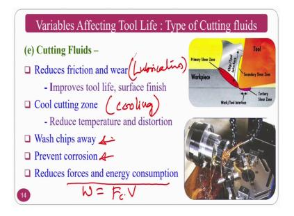
So, the cutting fluid basic function if you see that, it reduces the friction and wear and cools the cutting zone, that is nothing but cooling and lubrication this is called as lubrication, and this is nothing but cooling. So, 2 primary a functions of cutting fluid is cooling and lubrication, that is what I mean to say it from the first 2 points.
