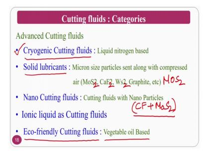
So, I am mixing and I am sending with high pressure what will happen? The density of particles is very high compared to my fluid. So, there is a tendency that in the chip tool interface, the particles will go and occupy this interior regions. So, that it may help in the lubrication also, at the same time it may try to lift by some of the nano meters or something.
