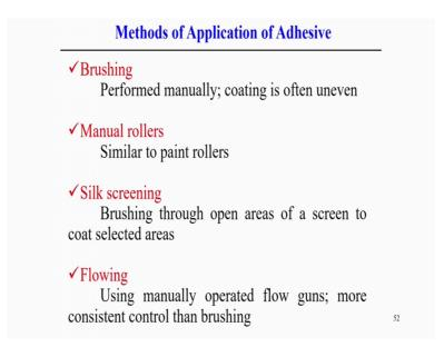
So, but now we come to that point that what are the typical methods of application of the adhesive? In what way we can put the adhesive between the substrate material? So, it simply manually we can do the simply brushing and, but when you do the manually this thing there is a possibility of the uneven coating; may not be the coating may not be the very even.
