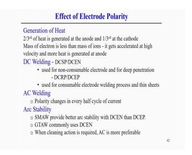
Now, when we use the electrical power source in case of the arc welding process so, basically there is a possibility of use. We can use the either direct current or alternating current, but point is that in the direct current there may be the possibility of the how to select the polarity of the electrode and the work piece. So, to understand the polarity of
