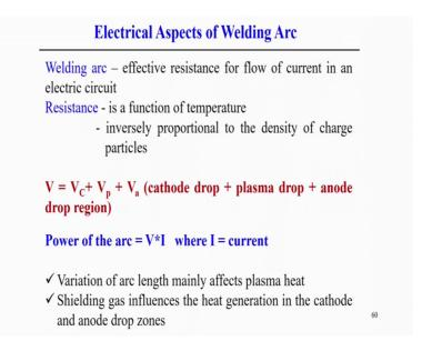
So, in terms of voltage drop we can find out the represent the electrical aspects of the welding arc in other way that welding arc can be represented that the effective resistance for flow of the current in an electrical circuit. So that effective resistance of the flow of the current in an electrical circuit and that how that flow of the electron; basically creates the amount of the heat either in the workpiece or either in the electrode material.
