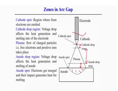
Now, if we look into the very intuitively that what are the different zone in the in a in a arc gap; we can find out that first is the cathode spot. So, that is a zone from other electrons are emitted emit electrons are emitted from the cathode. So, first the electrode is there and from electrode there is a then this component that is called the cathode. And the cathode drop zone these two certain zone from the cathode and this zone is basically called the cathode spot.
