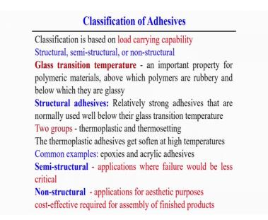
Now, classification of the adhesive what are the different different types of the adhesives can be used that are different way or different types of the adhesive materials can be used for the adhesive bonding, but here we try to do the classification based on the load carrying capability.
