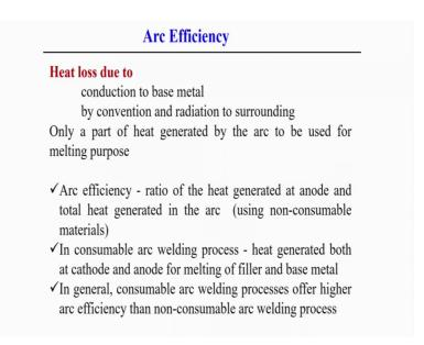
So, look into that that heat loss may be mainly due to the when application of the heat that comes from the creation of the arc; that one amount of the heat is conducted higher to the base material, but at the same time heat will heat lost due to the conviction and radiation from the work piece surface and that heat lost due to the surrounding.
