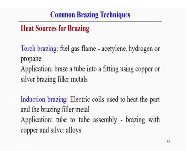
So based on that, we can define the different brazing techniques one is one is that torch brazing. So, in this case the fuel gas flame is basically used like acetylene hydrogen or propane they are used to heat the alloy material; braze alloy.
