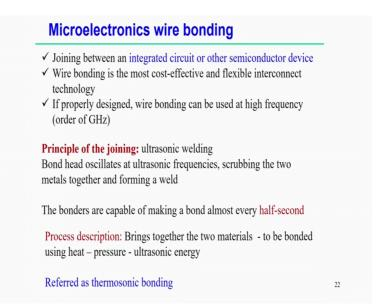
It is a joining between an integrated circuit or maybe other semiconductor devices, but in this case wire bonding is the most cost effective and flexible interconnect technology and, if you see that the wire bonding can also used even high frequency application of the order of the Giga hertz. But what are the principle of the wire bonding technology?
