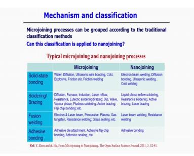
But question is that can this classification is applicable for nano joining processes? Let us see if you look into this table that typical micro joining and nano joining processes here if you see that solid state bonding, soldering brazing, fusion welding and adhesive bonding.
