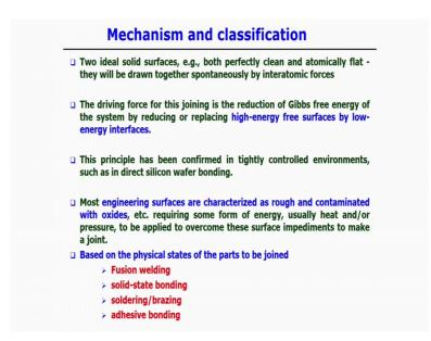
So, to start with that basic mechanism of the micro joining process or nano joining process maybe we can consider the 2 ideal surface both are perfectly clean that means, there is no oxide layer on the surfaces and they are atomically flat, atomically flat means if we see the under the at the scale of the at the atomic scale the surface should appears completely flat.
