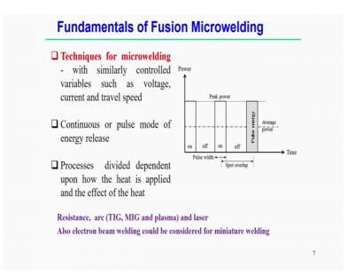
What are the different techniques for the micro welding processes? Already you described the different types of micro welding processes, but what are the basic needs for the development of the technology for the micro welding processes. So, first thing is that we need to control the different variables very precisely. Such as voltage currents and travel speed that also applicable in case of conventional welding processes, but still it is very much important in case of micro welding processes.
