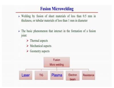
So, fusion micro welding probably we can define further that fusion micro welding process, when the sheet thickness of the materials is less than 0.5 millimeter, or maybe the tubular materials diameter is less than 1 millimeter in diameter, that can be considered as a fusion micro welding process. So, geometric size may be is restricting the definition of the micro welding process as compared to the conventional welding process.
