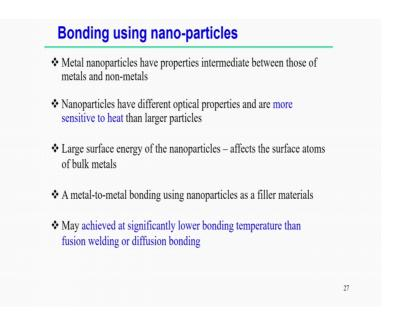
If we see that most of the nanoparticles maybe having the properties the intermitted between those of the metals and nonmetals, but nanoparticles having different optical properties and the more sensitive to the heat, than large particles large surface energy of the nanoparticles affects the surface atoms of the bulk metals.
