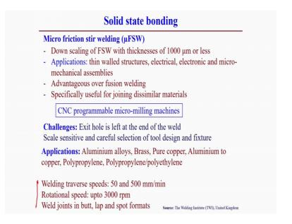
It is a simply down scaling of the friction stir welding process and we define the micro friction stir welding process, in terms of the thickness which is less than 1000 micrometer, or may be at the similar dimension. Typical application thin walled structure, electrical, electronics, micro mechanical assembly.
