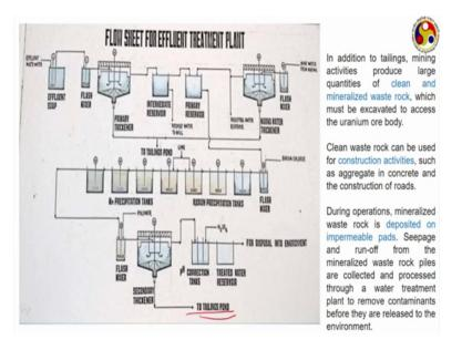
It is a possible flow sheet for this effluent treatment, they effluent that we are getting that goes to a series of reservers. Each of the reserver is own roll like a in this portion, radium is separated, amine is precipitation in this particular portion and Ph is connected in this particular tank. Accordingly, the effluent is allowed to go through series of chemical actions and so that finally, what comes out, what is going to the tailing ponds is
