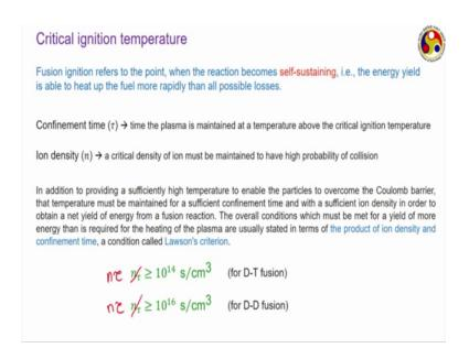
So, the temperature requirement is the biggest issue that we can have in order to facilitate the fusion reaction. We somehow have to produce that level of temperature and another issue is that whenever we reach that level of temperature all material turns to plasma.
