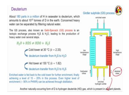
Here from the as the output from this cold reactor quite often is supplied back here or may be supplied to another reactor; which is placed in a cascaded position and we get repeated we get repeated enrichment. Similarly, this depleted water depleted here refers to the water which has transferred the deuterium to hydrogen sulfide thereby it is deuterium concentration has reduced.
