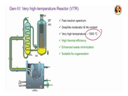
Very high temperature reactor, another concept again a fast reactor, it is an advanced version of the gas cooled reactors; It to the same graphite moderator and helium as the coolant, and can go up to extreme temperature of 1000 degree Celsius.
