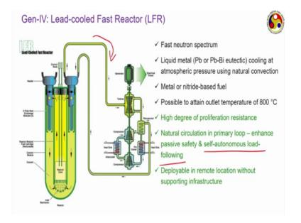
The second concept is lead cooled fast reactor. Again, it is a fast reactor, where we use some kind of liquid metal, liquid lead or lead bismuth eutectic mixture as the coolant. It works under atmospheric pressure, and makes big use of the natural convection. Then metal fuel or nitrate-based fuels are commonly used, and it can also go up to high temperature something like 800-degree Celsius.
