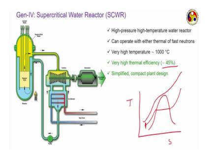
And finally, is the supercritical water reactor another novel concept. It uses high pressure high temperature water reactor. As the name suggests is supercritical that is the water that we use here as coolant that works at a condition beyond it is critical point. I hope you remember that the critical pressure for water is about 22.1 mega Pascal and a critical temperature is 374-degree Celsius.
