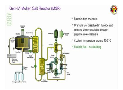
Molten salt reactors again is fast reactor, which uses uranium fuel dissolved in some kind of fluoride salt coolant which circulates through the graphite core channels. It attends slightly lower temperature compared to the previous to something in the range of 700degree Celsius. And a big advantage is the flexibility in the form of fuel that we are using as we are a using a fuel dissolved into a coolant. So, no cladding is required, and we can use different kinds of fuels.
