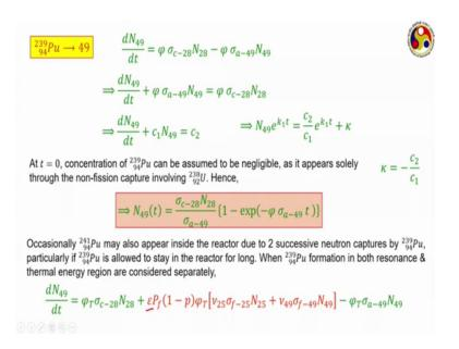
Next, we move to plutonium, plutonium as a short for notation is 49, this is a corresponding conservation equation there are 2 terms. This is the decay rate of uranium 238, because of which is plutonium is getting formed, and this is the dk rate of plutonium itself.
