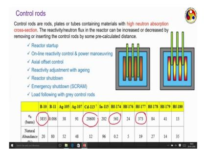
And the most common one of them is the control rods. Control rods are some elements which can be of the shape of rods or plates or tubes which contains materials which has very high absorption cross section.
