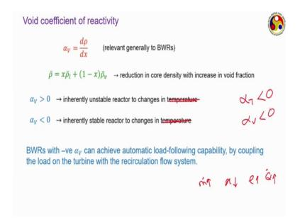
Therefore we have seen the temperature coefficient of reactivity should be negative for a stable operation. Similarities void coefficient of reactivity should also be negative. The boiling water reactor is negative alpha v we can achieve automatic load following incapable, because just the way I have mentioned. They couple the load on the turbine with the recirculation flow systems.
