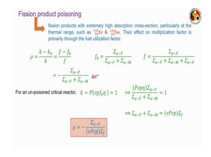
Let me go through quickly to the last part of this particular module, where we shall be discuss about fission product poisoning. Poisons refers to certain isotopes which may appear following radioactive decay of the fission products, which is extremely high absorption cross section. Like, xenon 135 and samarium 149.
