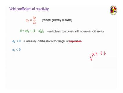
Similarly, when alpha v is less than 0, in that case, when x increases rho, reduces as the rho is reducing, then corresponding power production from the reactor also reduces. Hence lesser amount of energy is transferred to the moderator. They were reducing the total void generation, and that therefore, tries to reduce this x itself acting like a feedback mechanism.
