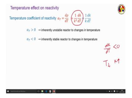
We can we will study the other case also. Like, if there is a reduction in the temperature. Any temperature reduction will cause on increase in the reactivity, and once the reactivity increases. So, the power produced by the fuel pins that will increase. So, that will try to increase the temperature level of the reactor, and here the temperature will try to get back to it is original value thereby restoring the reactor back to it is initial position.
