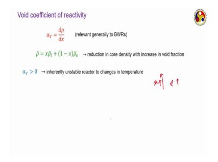
There is another effect the void coefficient of reactivity, which actually refers to the rate of change of reactivity with x, x is called void fraction, void fraction can be defined as the volume fraction of the vapor phase in a mixture of liquid and vapor.
