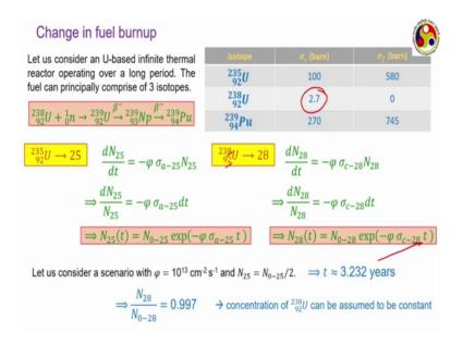
So, this is the corresponding equation uranium 235 there is no source of production, but it decays by absorption of neutron. And then we rearrange the equation, and we get this exponential solution.
