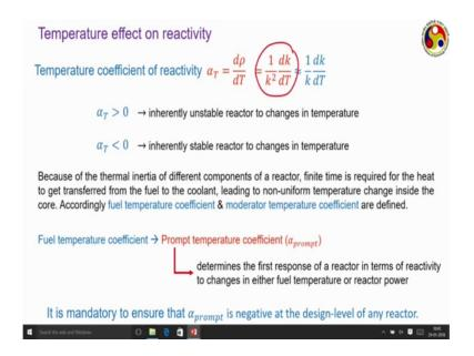
Generally, because of the thermal inertia of the different components of reactor the temperature inside is not uniform. Like, whenever there is a change in the reactivity is the fuel pin whose temperature increase first. Then that temperature will be transferred to the cladding that energy will get trans transfer to the cladding and from cladding to the coolant or to the moderator. And this entire energy transmission process it may require some finite amount of time
