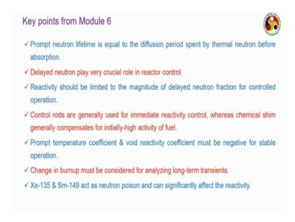
We have discussed about the role of control rods and chemical shim etcetera; control rods are generally used for immediate reactivity control. Whereas, chemical shims generally compensate for initially high activity of fuel, or for slow control chemical shim can be used. Then we have discussed about the effect of fuel burn up, the effect of temperature we have discussion the prompt new temperature coefficient and void reactivity coefficient both should be negative for stable operation.
