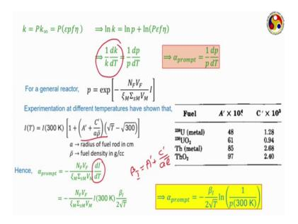
Let us see mathematically the effect of this and Doppler reactivity, we know from the definition of multiplication factor it is the product of p into k infinity. The k infinity is the infinite multiplication factor and p is the total non-leakage probability, which combines both first and thermal non-neutral non-leakage probability normally.
