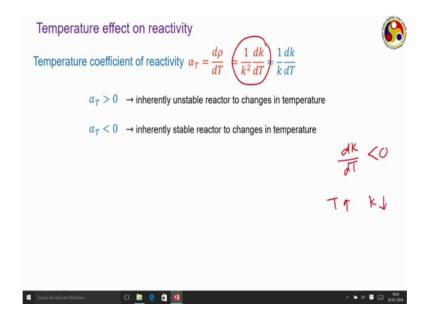
Which is a very much undesirable situation; so, the reactor is inherently unstable with changing temperature.
