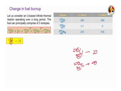
Next let us check the effect of fuel burn up, we have seen the effect of temperature now fuel burn up or the change in the fuel fraction inside the reactor. Let us consider an infinite thermal reactor which is operating based upon uranium. Now, we remember that you natural uranium generally comprises of three different isotopes; Uranium 235 about 0.7 percent, uranium 238 99.3 percent and very stress quantity of uranium 234.
