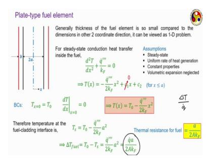
Now, resistance can be defined as the drying force for the heat transfer which is the temperature difference across the fuel divided by a heat transfer rate; that is delta T by q dot and accordingly the thermal resistance for the fuel is a by 2 capital A into k F.
