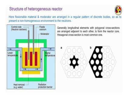
In heterogeneous nuclear reactor we have mod material the fissionable mixer; that is fuel and moderator keep separately, but they generally add in this some kind of regular pattern some kind of repeatable regular pattern and very fuel component is internally separated by a moderator with the adjacent fuel components just a represent picture like this here the red o blocks are actually fuel which are surrounded by moderator this yellow colored one from all possible sides.
