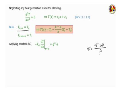
Now, we move to the cladding there is no heat generation inside the cladding and hence a we have a very simple form of homogenous second dot dot d whose solution will be c 3 x plus c 4 for x equal to a to b.
