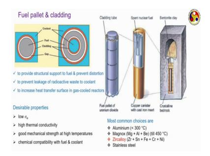
Then we come to fuel pallet and fuel cladding pallet refers to each small module of fuel element which can be of the shape of small bullets or may be a just like a small tablet and their covered by a jacket which is called cladding claddings of several important purpose like; a this is a much elaborated diagram where you can clearly see each of the module here like this is the one this one is the fuel module and this module is being covered by the cladding material.
