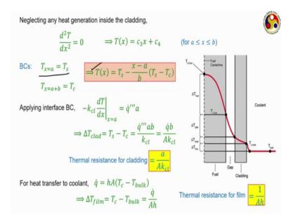
And subsequently we get the temperature change across the cladding; that is, T s minus r c should be of a form like this q dot b by A into k c l.
