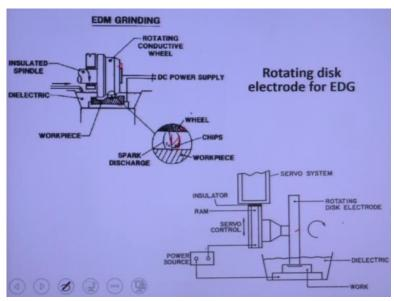
So here you can see this is the rotating grinding wheel, graphite grinding wheel is there. So this is the workpiece and you can see this is the sparking occurs. After sparking these are the debris particles, which is flushed away on the interelectrode gap by the rotating grinding wheel. So this wheel actually it is a graphite. It is a conducting material, conducting material, graphite is used. So you can see here this rotating electrode disk is there.
