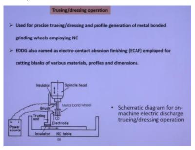
So this trueing and grinding operation using this electrodischarge diamond grinding you can prove, you can do the trueing operation or dressing operation. So used for precise trueing or dressing and profile generation of metal bonded grinding wheel employing this NC concept. Electrodischarge diamond grinding also named as electro-contact abrasion finishing, electro-contact abrasion finishing, ECAF employed for cutting blanks of various materials, profiles and dimensions.
