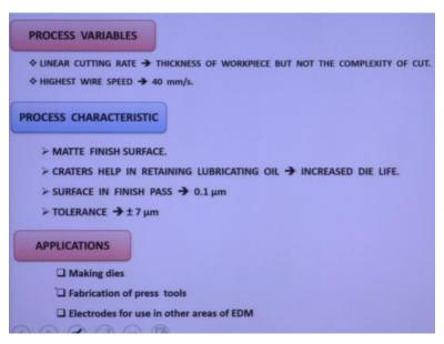
So this process variables, linear cutting rate. It depends on the thickness of this workpiece material but not on the complexity of the cut. So it depends, this linear feed rate of this wire, it depends on the thickness of this workpiece material. So highest wire speed is 40 mm/s. So process characteristics because of this craters generated because of the sparks craters are generated on the workpiece surface, this matte finish is actually generated.
