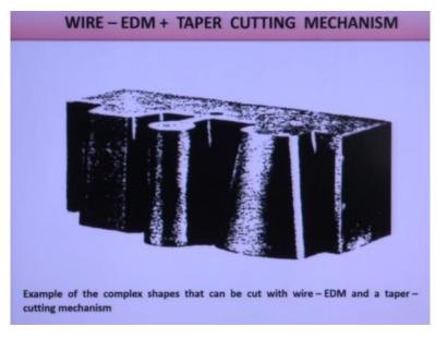
This is the example of complex shape that can be cut with a wire EDM and taper cutting mechanism. So this kind of inclined surface can be generated by a tilted wire in wire EDM process. So now we shall start with electrodischarge grinding. So grinding we know this conventional grinding process there 1 grinding wheel where this abrasive particles are bonded. So this grinding operation can be conventional grinding or hybrid grinding but in hybrid grinding
