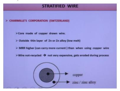
So there is a concept that is called this stratified wire. In stratified wire this core material is made of copper and the outer material is made of this zinc and zinc alloy. So this core material is made of copper drawn wire and outer thin layer is made of zinc and zinc alloy which has a low melting point than the copper. So if we need high material removal rate it should carry more current than
