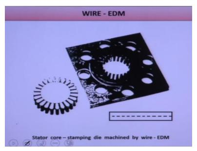
So you can see this kind of stator for the motor is can be made, this kind of complicated surface on a 2D complicated surface can be generated so which is used for this stator core is the stamping die machined by this wire EDM okay, can be machined by the wire EDM this kind of complex contour on a 2D surface can be generated by wire EDM process.
