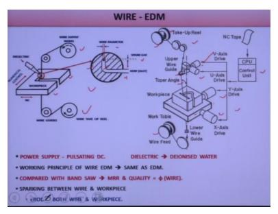
So first one is the your power supply DC power supply, pulse DC power supply is the first one. So DC power supply then air positioning system is there second one, then dielectric system is there and then wire drive system is there. So these are the 4 important components of wire electrodischarge machining process.
