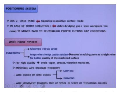
Now third component of the wire EDM process is positioning system. So these wires has to be positioned very accurately because we are going to cut a very complicated surface or contour from the workpiece surface. So using a CNC controlled 2-axes, 2-axes controlled table we can use, we can use a 2D complicated surface we can use.
