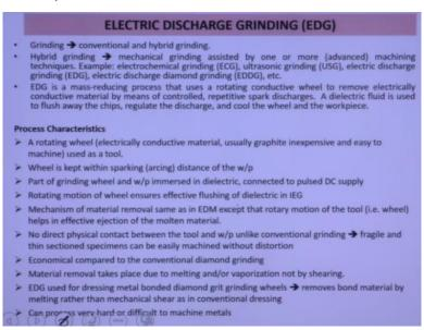
So this electrodischarge grinding also hybrid grinding operation. So it is a mass reducing process that uses a rotating grinding wheel to remove the electrically conductive material by means of a controlled repetitive spark discharges. A dielectric fluid is used to flush away the chips, regulate the discharges and cools the wheel and the workpiece. We know that in normal EDM operation so there is a very problem of the dielectric flushing system.
