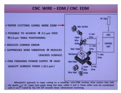
So this is the CNC wire EDM system. You can see here V axis, U axis is there. So taper cutting can be done using this wire EDM, the CNC wire EDM. Possible to achieve 0.1 micron feed and 1 micron table positioning is possible and it reduces the corner wire, corner error. Suppresses the wire vibration and reduces the cracked surface. Fine finishing power supply quality surface is less than 0.1 micron.
