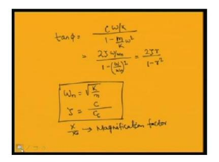
X by X 0 is known as the magnification factor of the system, and we can plot. So, this is magnification factor. So, one can plot this magnification factor versus the frequency ratio of the system. So, from this equation you can see that when r equal to 0 that is when omega equal to 0. So, this becomes 1. So, r equal to 1. So, this becomes 2 zeta. So, this is when r equal to 0. So, this becomes 1 and this part equal to 0. So, this is 1 by 1. So, this becomes 1.
