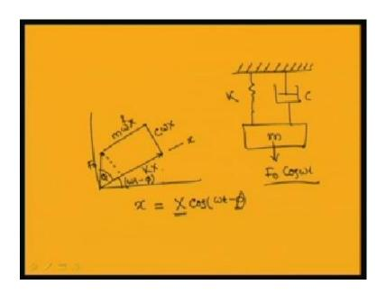
And in this graphical method I have taken the force polygon by drawing the forces, the spring forces, damping forces and the inertia force. And I have found the response of the system by drawing a line parallel to this damping force and forming a right hand triangle. So, in this right hand triangle I got this square plus this square equal to four square. So, I got the response of the system.
