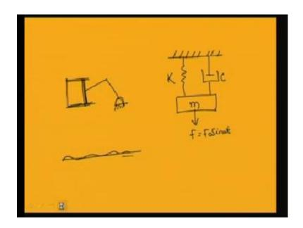
And in some cases like in case of the reciprocating engine or in a vehicle moving on the road; so some force is transmitted to the system itself. So, due to the transmission of this force or due to these forces, the system is subjected to forcing. So, this force may be of different types.
