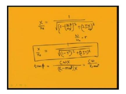
So, this displacement X can be given by. So, this X can be given by this or X by X 0 can be given by 1 by root over 1 minus omega by omega n whole square plus 2 zeta omega by omega n whole square. So, I can write this omega by omega n equal to r, frequency ratio. So, this equation I can write equal to. So, this will be equal to 1 by root over 1 minus r square whole square plus 2 zeta r whole square.
