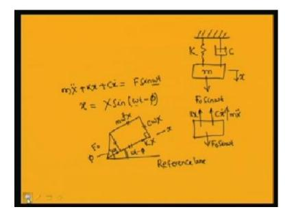
Now I have to find the phase angle. So, this phase angle phi also can be obtained from this triangle. So, in this triangle this tan phi will be equal to c omega X by k X minus m omega square X. So, I can write tan phi equal to c omega X by k minus m omega square X. So, cancelling this X X, it is equal to c omega by k minus m omega square. So, again now dividing this k in the numerator and denominator I can write this equal to.
