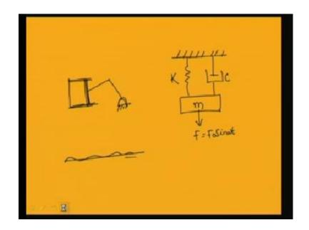
So, let us take a simple spring mass damper system. In the simple spring mass damper system which is the model of most of the systems, you can write the mass equal to m, spring stiffness equal to k, and c is the damping. It is subjected to a force F equal to F 0 sin omega t. So, this simple model can be a model of an IC engine or reciprocating engine. In case of a reciprocating engine you know that the unbalance force always there is the presence of an unbalance force.
