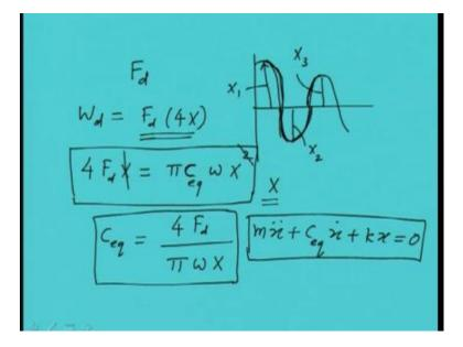
So, as we know that the damping force remains the constant and when we are talking about the motion decaying, this is the decay, and let us say this is the x 1, this is x 2 and
