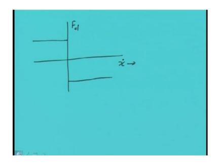
Now let us see how this particular friction force changes with speed as we know that when body starts moving it. So, if we have positive display or positive velocity, the force will be acting in the negative direction like this. And when body is going in the opposite direction that is toward the negative, it is having negative velocity, then we will be having force here. So, we can see that they are constant but changing depending upon the direction of velocity.
