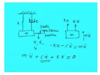
So, for this let us take a simple model in which we have one spring and mass, and apart from this. Now we are attaching one damper also. So, damper we represent like this in which this represent some kind of piston. This is cylinder and ceases the damping coefficient. K is the stiffness of the spring and mass m, and here let us say this is again static equilibrium position of the mass. So, when we are taking the reference as the static equilibrium position, the gravity effect will not come.
