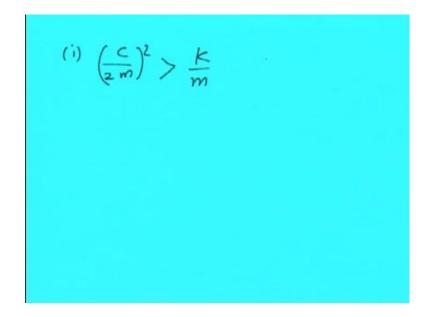
So, first case when within this square bracket this term, or I should say this quantity is greater than k by m. So, that means within the square root we will be having positive quantity.
