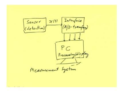
So, in measurement system we have a sensor which detect the vibration is the detection of the vibration and it gives in the form of displacement with respect to time then we have, the interface which converts the analog signal which is measured by the sensor to the digital form A to D transform. Then we feed this to this signal the digitized signal to a personal computer and there we do the processing of the measured signal processing and display of the signal.
