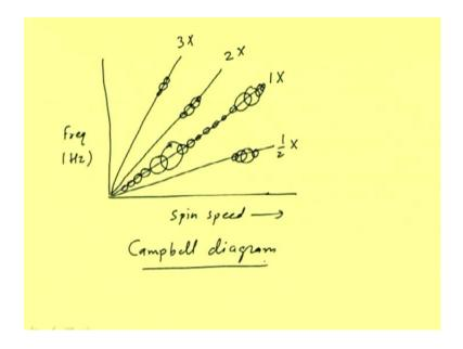
We can have like, this is a Campbell diagram in which this axis is spin speed and there is the frequency of the vibration which is in Hz. Now, we have this line which is corresponding to the rotational frequency component and some more components are there which are twice the rotational frequency or may be 3 times the rotational frequency or even we can have half the rotational frequency components.
