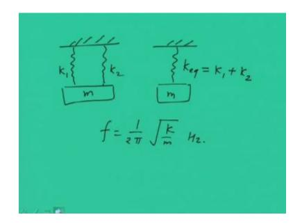
And, if we have another system in which springs are connected like this - K 1 and K 2' mass is here. So, in this particular case, also, we can have an equivalent system with K equivalent; where K equivalent now will be given as summation of these two, because they are connected parallel. So, same equation is valid here also, that is, in hertz.
