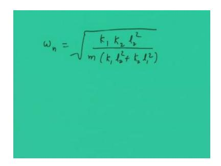
So, natural frequency of the system will be this. So, you can see that, here we have not obtained the free body diagram of this member. But, directly we obtained how much static deflection of this particular mass is taking place. And based on that, we could able to get the natural frequency of this system.
