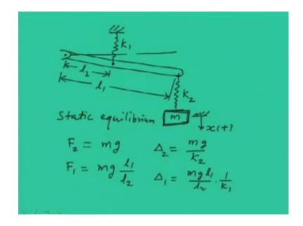
To have better understanding of how to obtain the natural frequency of a particular system, especially for single degree of freedom system; now, I will be taking another example. The example is in which we have one rigid member like this. At the end of that, one spring is attached and mass is suspended. The stiffness of this is K 2. There is another spring here having stiffness K 1. The length of the rod from here is 1 2. And total length is 1 1.
