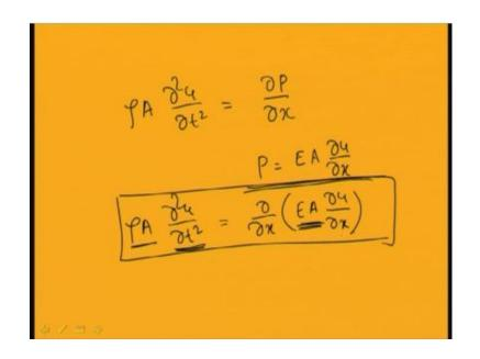
Del square u by del t square is the acceleration rho A is the mass. So, mass into acceleration this is the inertia force or the force acting on the system.
