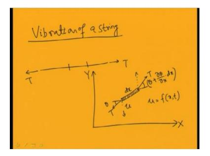
At this point is nothing but this is the differential of this deflection at that point. So, deflection is u, so the slope will be equal to...
