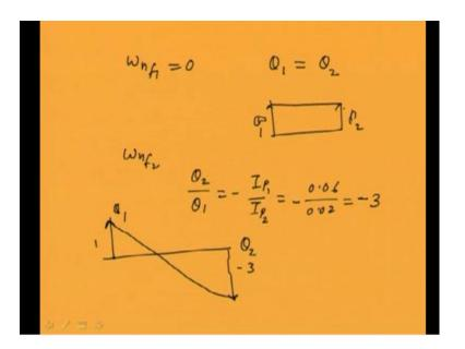
Now, let us see the modes shapes corresponding to the first natural frequency will be having both the displacement same. So, mode shapes remains like this, both are same theta 1 theta 2. Corresponding to the second natural frequency; will be having mode shape which is 0.06 by 0.02 minus. So, it comes out to be minus 3. So, the mode shape will be something, if we have 1 here, second will be having minus 3 displacements. So, this is corresponding to the second natural frequency mode shapes.
