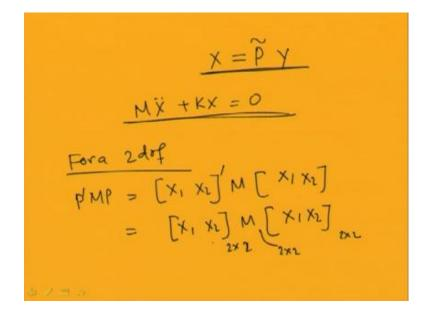
So, if I am assuming this uncoupled mass principle coordinate is Y. So, I can substitute this X given the coordinate system X Y can use this X equal to P weighted modal matrix Y. And, I can also decouple this equation motion M X double dot plus K X equal to 0. So, before decoupling this thing; let us see some of the properties of this weighted modal matrix and modal matrix. Let us see one example; so for a 2 degree of freedom system.
