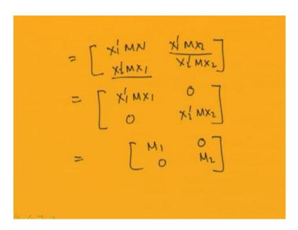
And, this P dash M P I can write equal to, so this will be equal to X 1 dash M X 1 X 2 dash M X 1 X 1 dash M X 2 and X 2 dash M X 2. So, now using this orthogonal property I can write this X 1 dash M X 2 equal to 0, and X 2 dash M X 1 equal to 0. So, this becomes X 1 dash M X 1 0 this is 0 and this is X 2 dash M X 2. So, this is equal to the generalized mass matrix M 1 0, 0 M 2.
