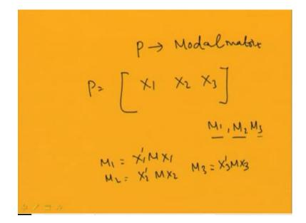
So, let modal matrix is P, so P is the modal matrix the weighted modal matrix can be obtained by dividing the. So, let P matrix let me write it equal to X 1 X 2 X 3 for a 3 degree of freedom system. And let M 1 M 2 M 3 are the generalized mass. So, M 1 can be obtained from these. So, M 1 equal to X 1 dash M X 1, and M 2 equal to X 2 dash M X 2 and similarly, M 3 equal to X 3 dash M X 3.
