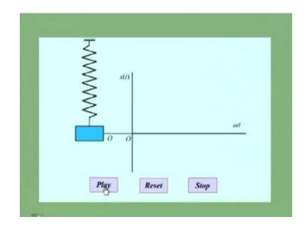
This is a spring mass system. The mass is... It is equilibrium position – static equilibrium position. And now we are giving a disturbance to this mass and we will track the displacement of this with respect to this time; this is time.
