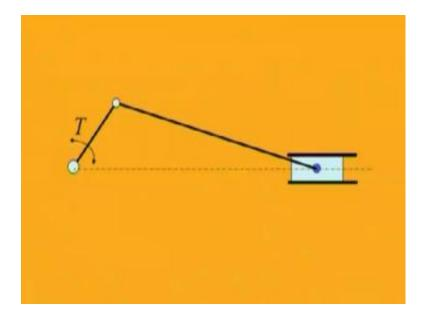
So, this is the schematic diagram of a slider crank mechanism usually used IC engine or reciprocating engines. So, in that case due to the unbalance forces or due to the forces of the piston. So, there will be an unbalance force always there is a unbalance force which cause the shaking moment, or shaking force which is also known as shaking force at the
